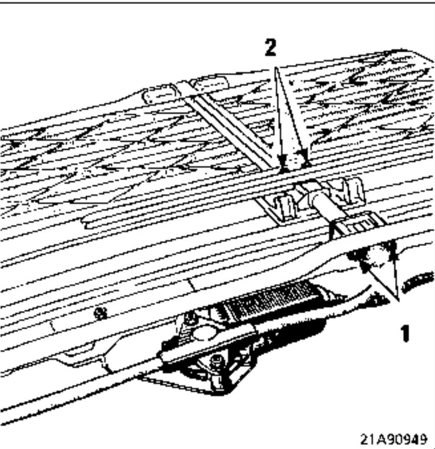
Remove the 2 nuts (1) securing the control cable sheathing to the rain channel.
