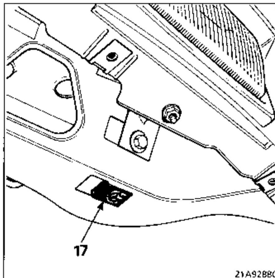
Fit the sheet metal nuts (17) to the front lower cross member
