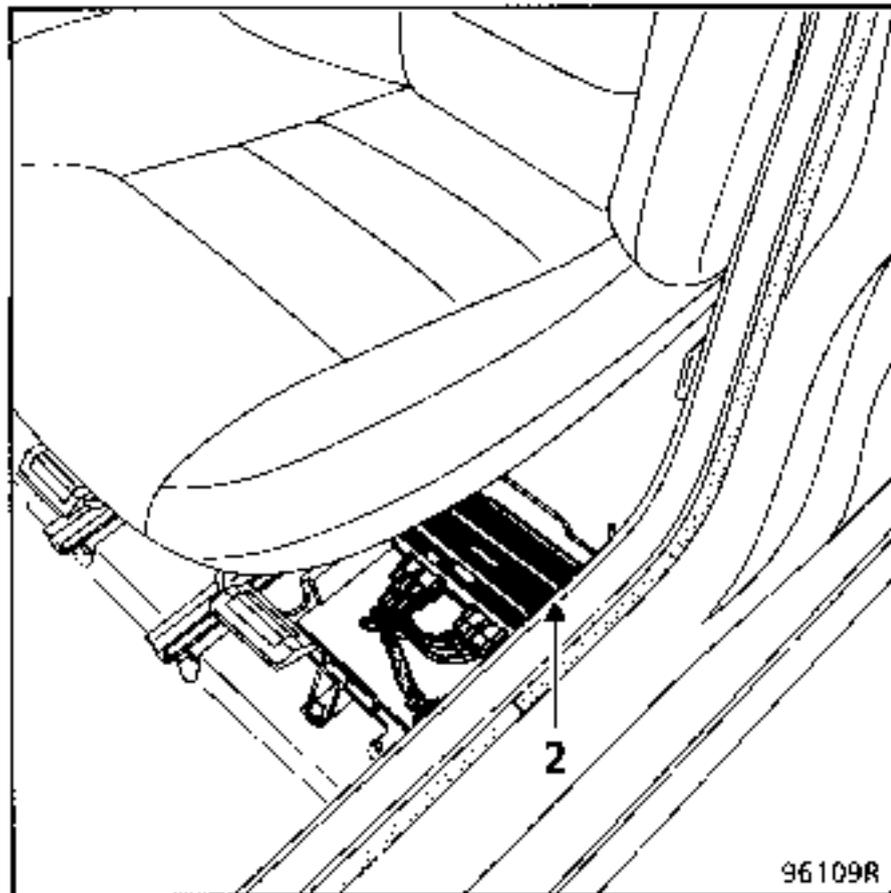
**WARNING :** For replacement of the decoder unit, refer to Section 82.
