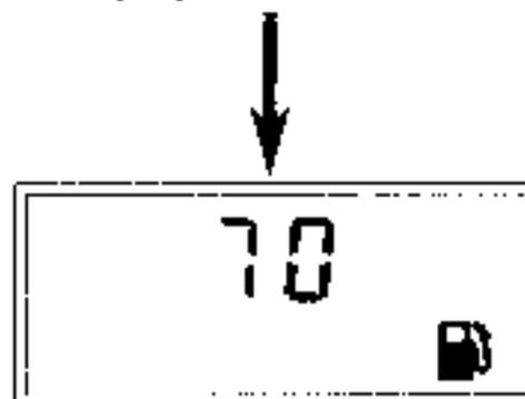
It is an indication that there is a short-circuit on the tank unit or its wiring.
