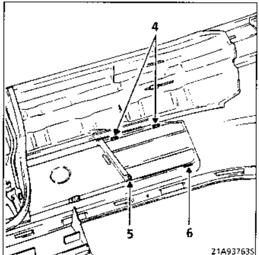
The front bumper supplied by the Parts Department comes fitted with 2 clips (4) which are used to secure the blanking cover (1) or the grille (2).
