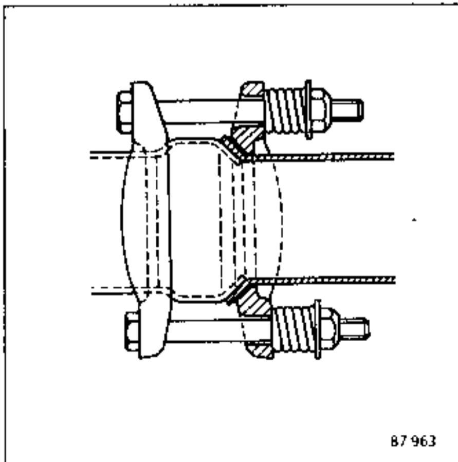
The joint is sufficiently tight as soon as an effective seal is obtained between the two pipes.
