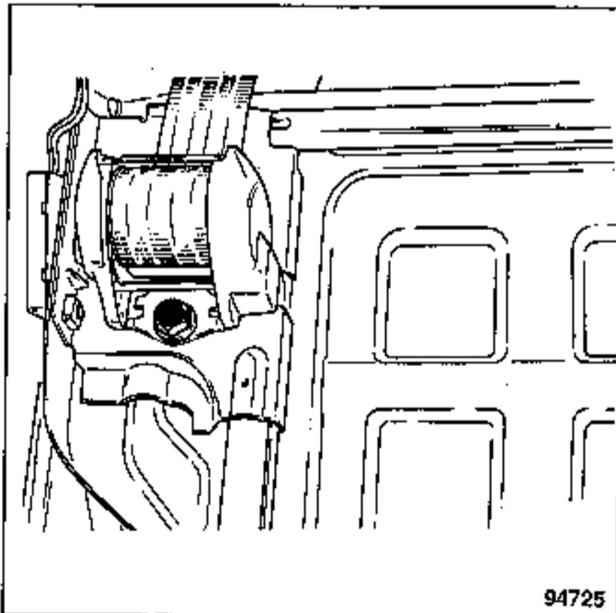
After stripping the seat back, remove the seat belt mounting.
