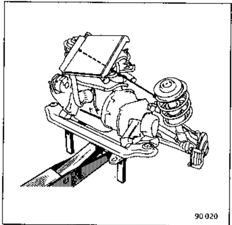
Secure the spring-shock absorbers in place with the string.
