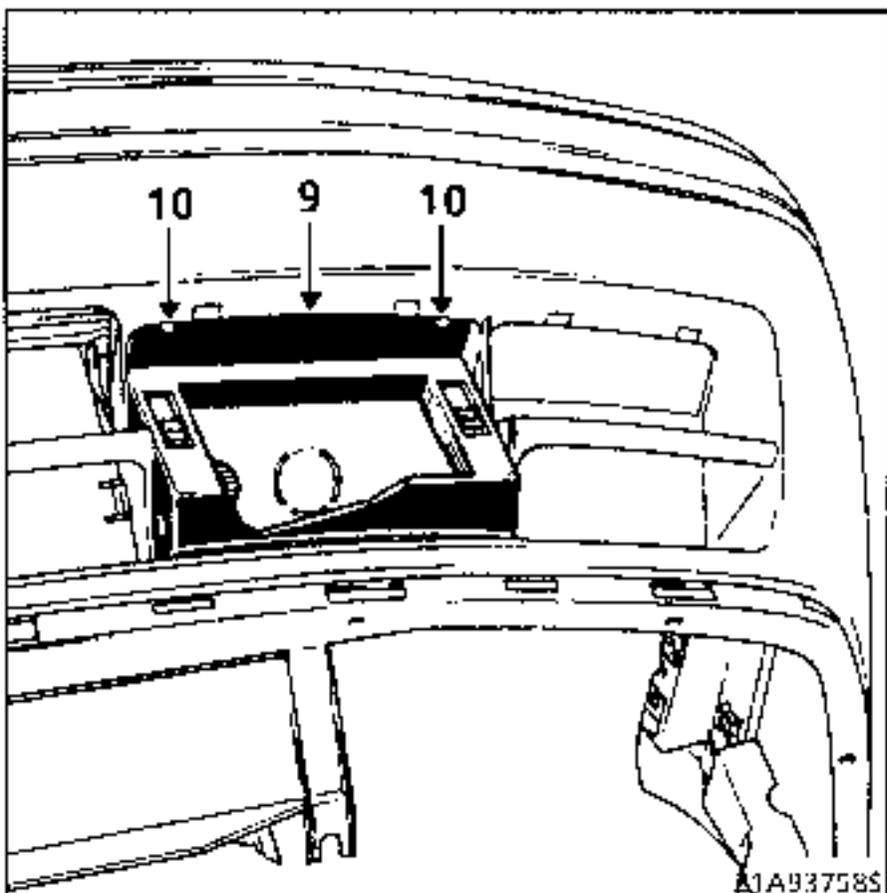
Clip the empty light bracket (9) into its fitting location.
