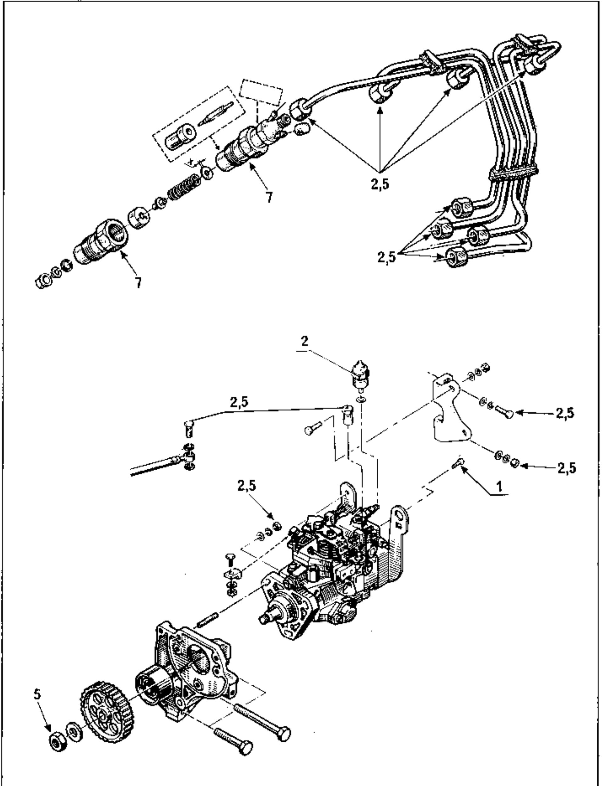
EXPLODED VIEWS - TIGHTENING TORQUES (in daN.m)
