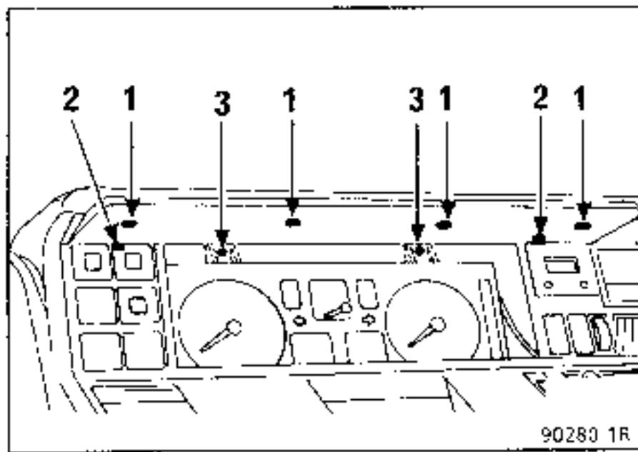
Disconnect the speedometer drive cable through the fuse box access panel.
