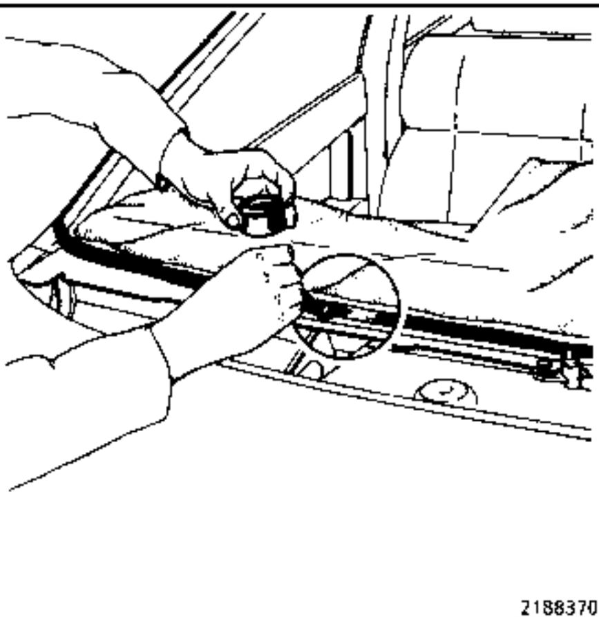
Apply metal primer to those areas where the surround has been stripped back to the bare metal during removing or cleaning operations.
