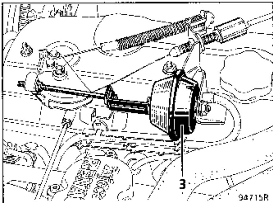
The valve acts on the throttle control in parallel with the pedal control.
