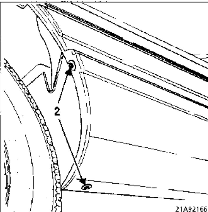
On the left-hand and right-hand sides, remove the two bolts (2) securing the plastic protectors for the wheel arches.
