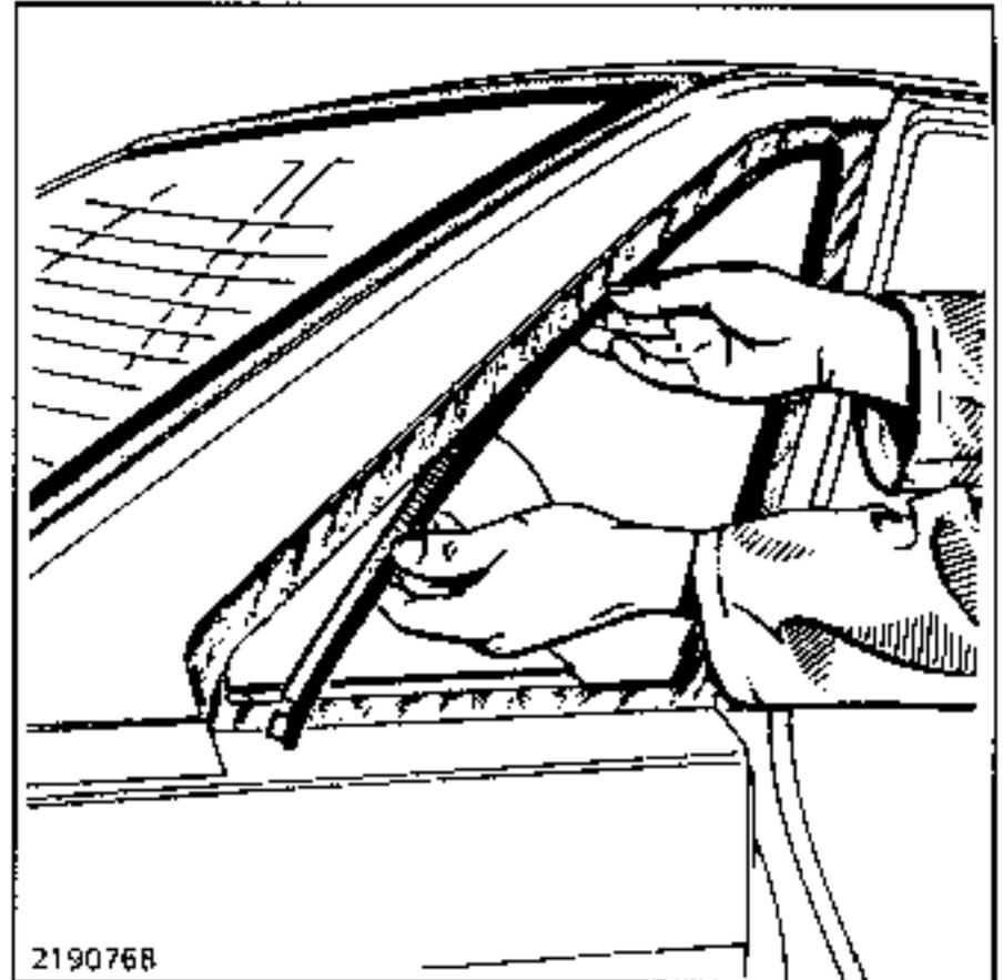
Fit the anti-overflow seal, bonding the adhesive surface inside the aperture.
