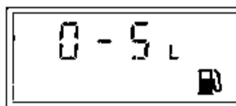
But the tank is not empty, there is a short-circuit on the tank unit or its wiring.
