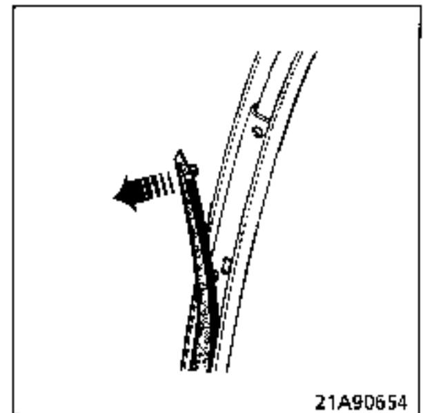
The plastic sheet is removed by cutting the mastic using a blade.
