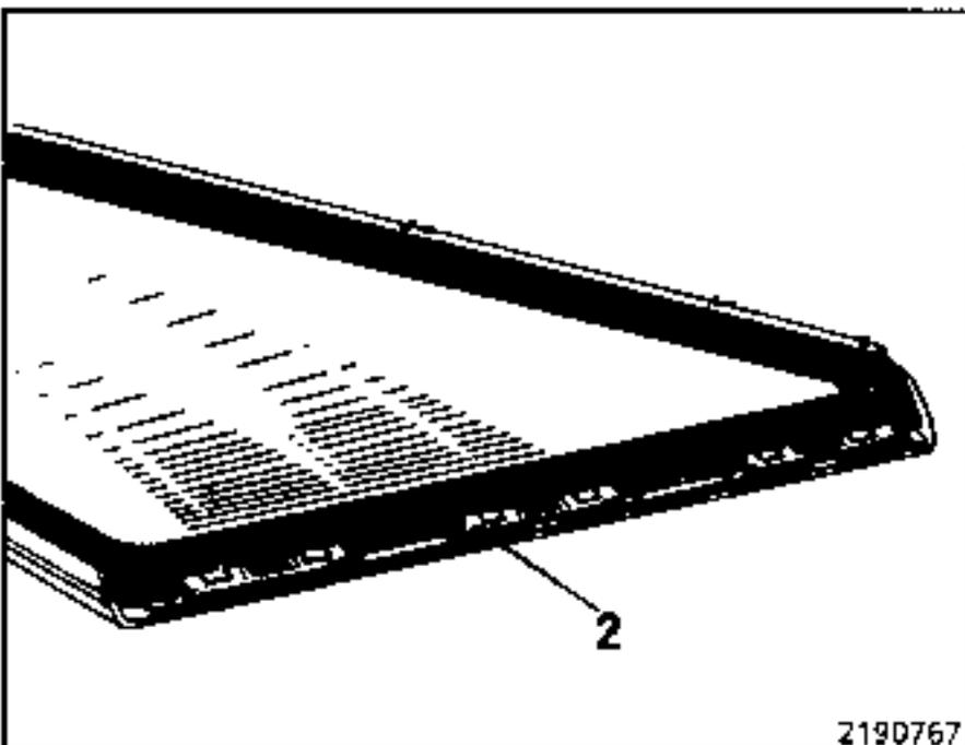
fit the clips (2) securing the moulding frame to the glass.
