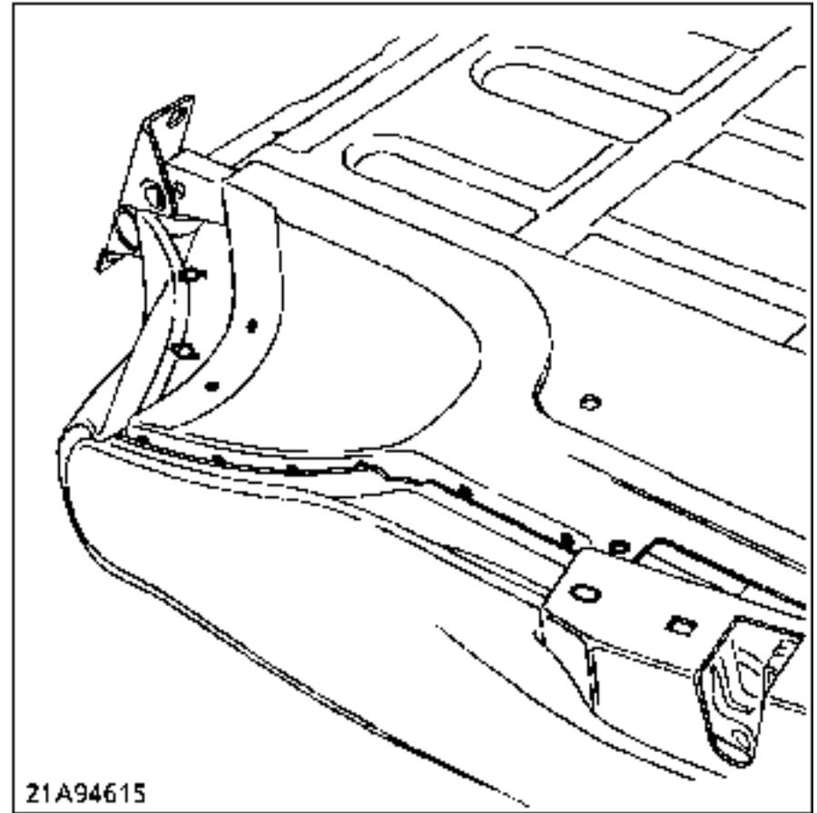
Remove the rear cover ("fir tree" type clips).
