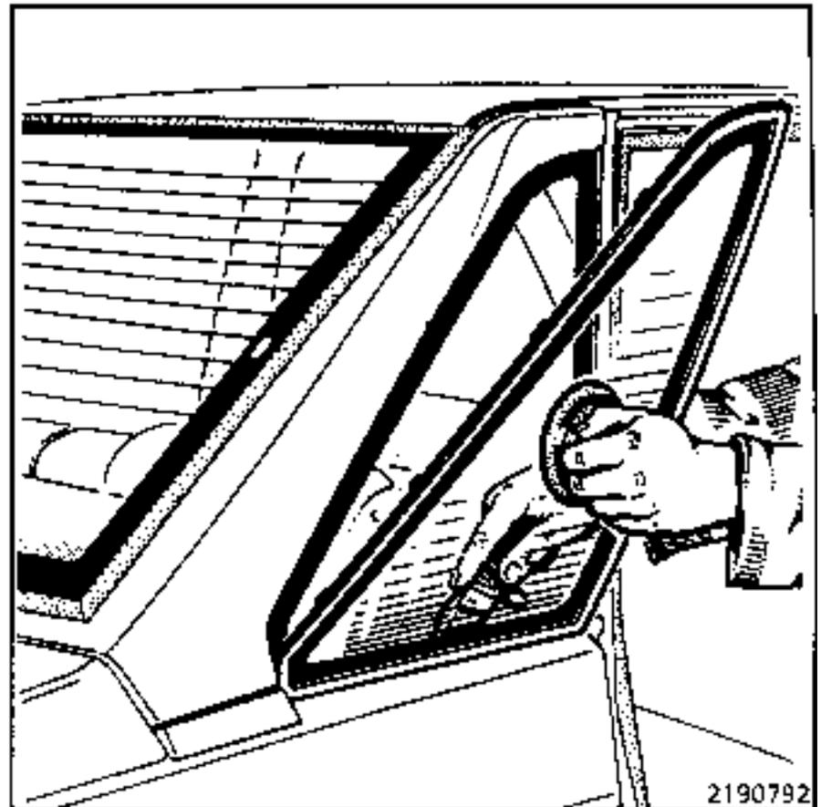
After cutting the first 2 sides, move the window away and, using a sharp blade, cut the remaining mastic taking care not to catch the 3 clips holding the frame.
