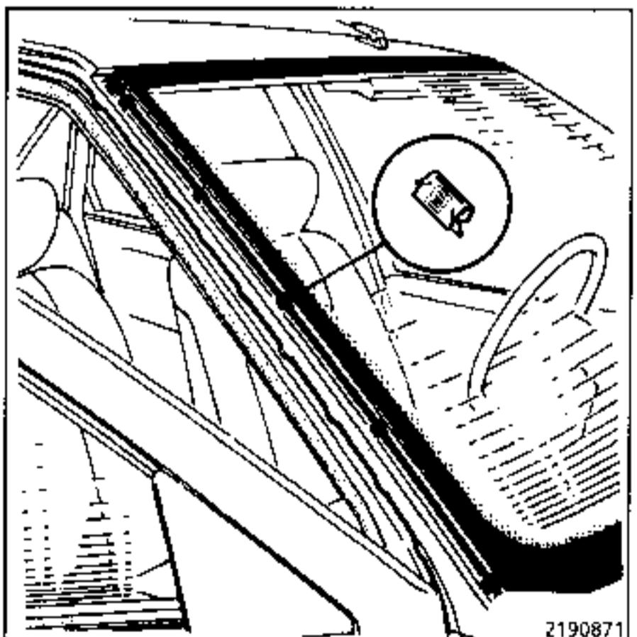
When the mouldings have been removed, 6 holding clips should remain on the aperture in the positions shown in the drawing. If necessary, replace any missing clips (direct the clips so that the spikes are facing outwards).
