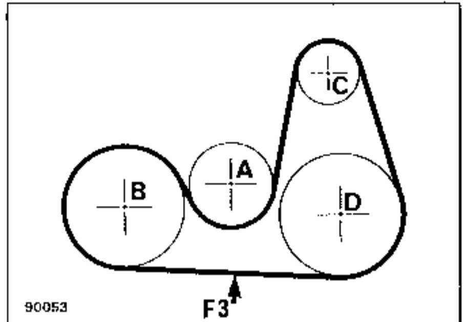
Coolant pump-Power steering- alternator belt
