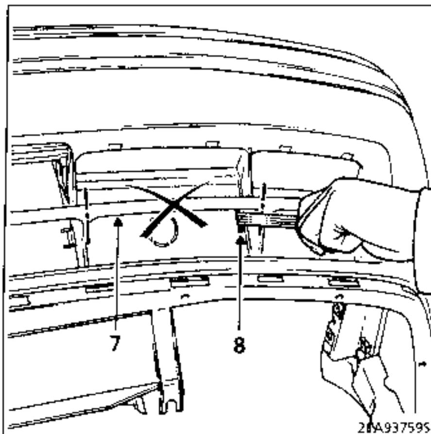
Using a hacksaw blade, cut the plastic bar (7) making use of the two oblong holes (8) situated at the bottom of the fitting location.
