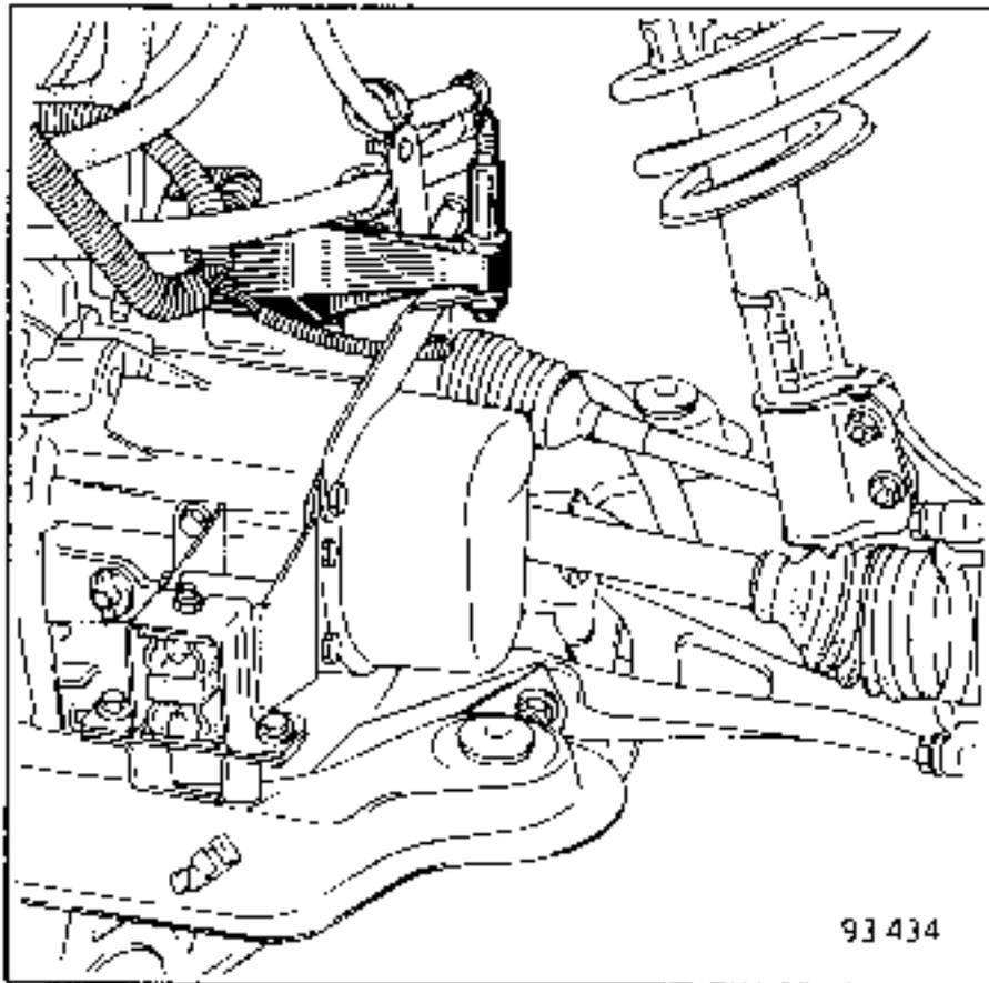
Lift the vehicle body and take out the power unit assembly.
