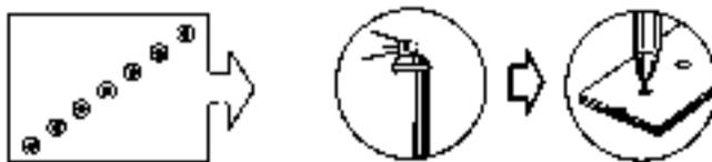
Nine plug welds (drill to diameter 6.5 mm).
