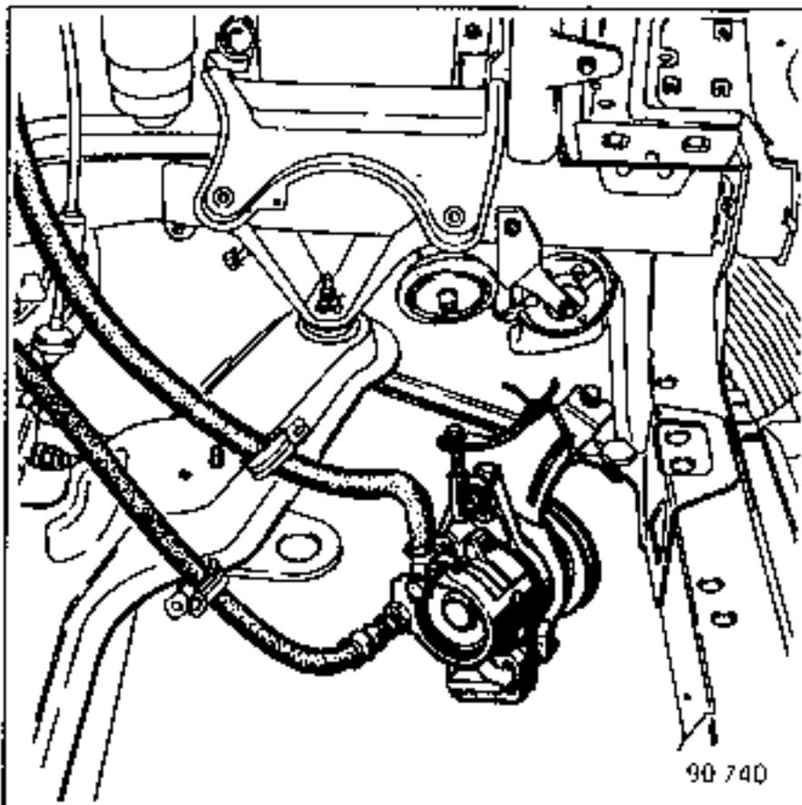
After fitting the power steering pump, check the drive belt tensions using tool **Ele.346-04**.
