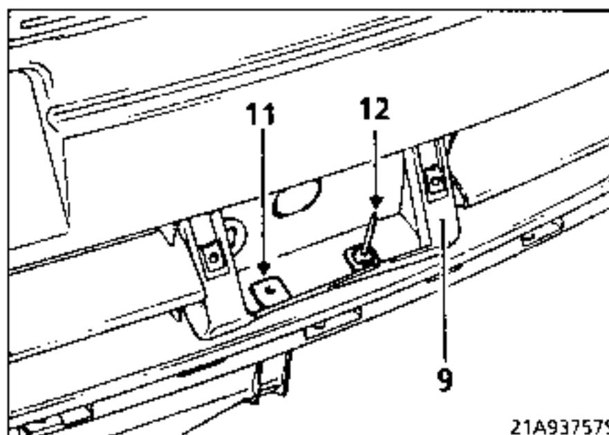
Mark the position of the two lower securing points (11) on the bumper.
