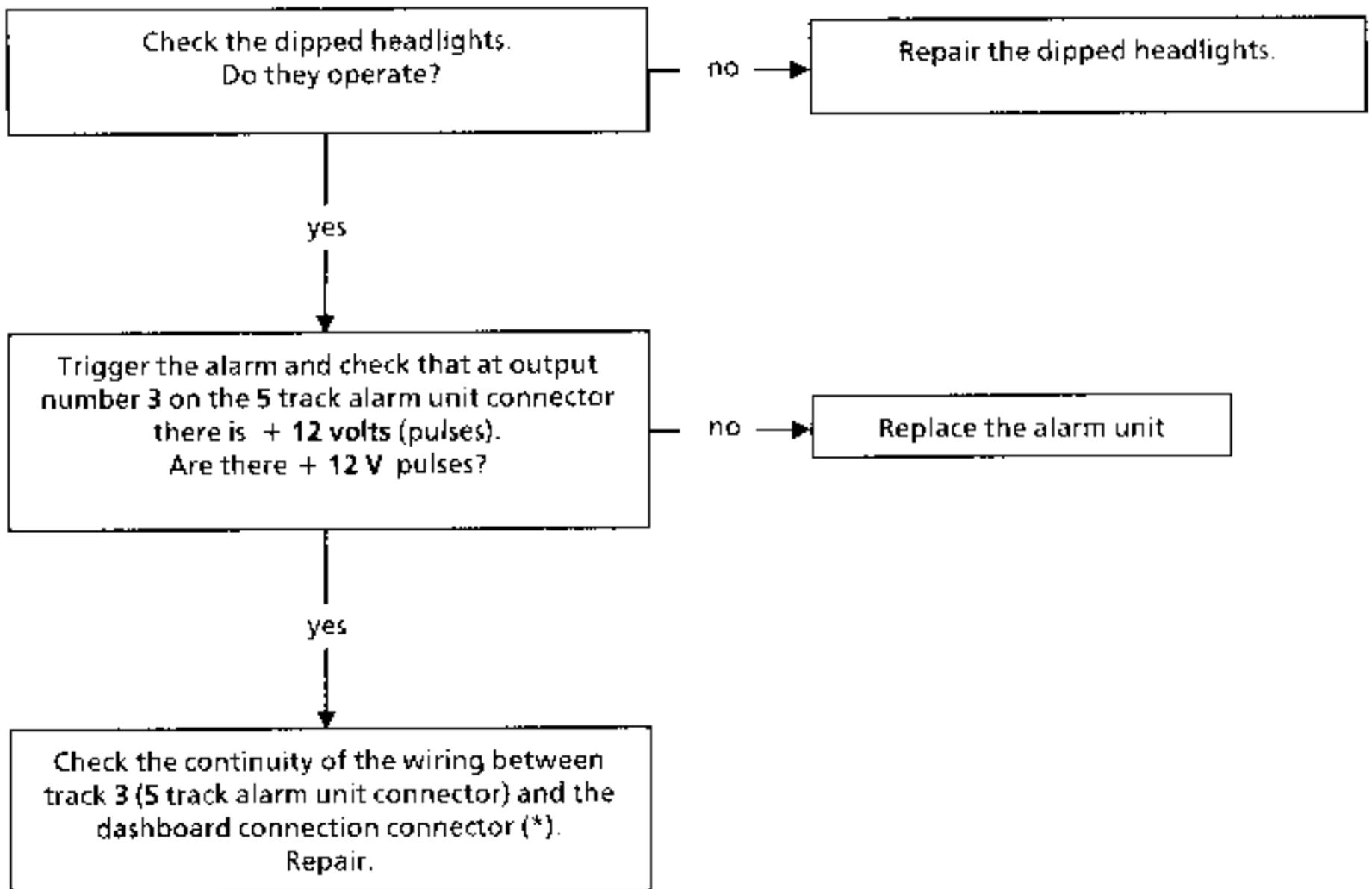
(\*) see vehicle wiring diagram
