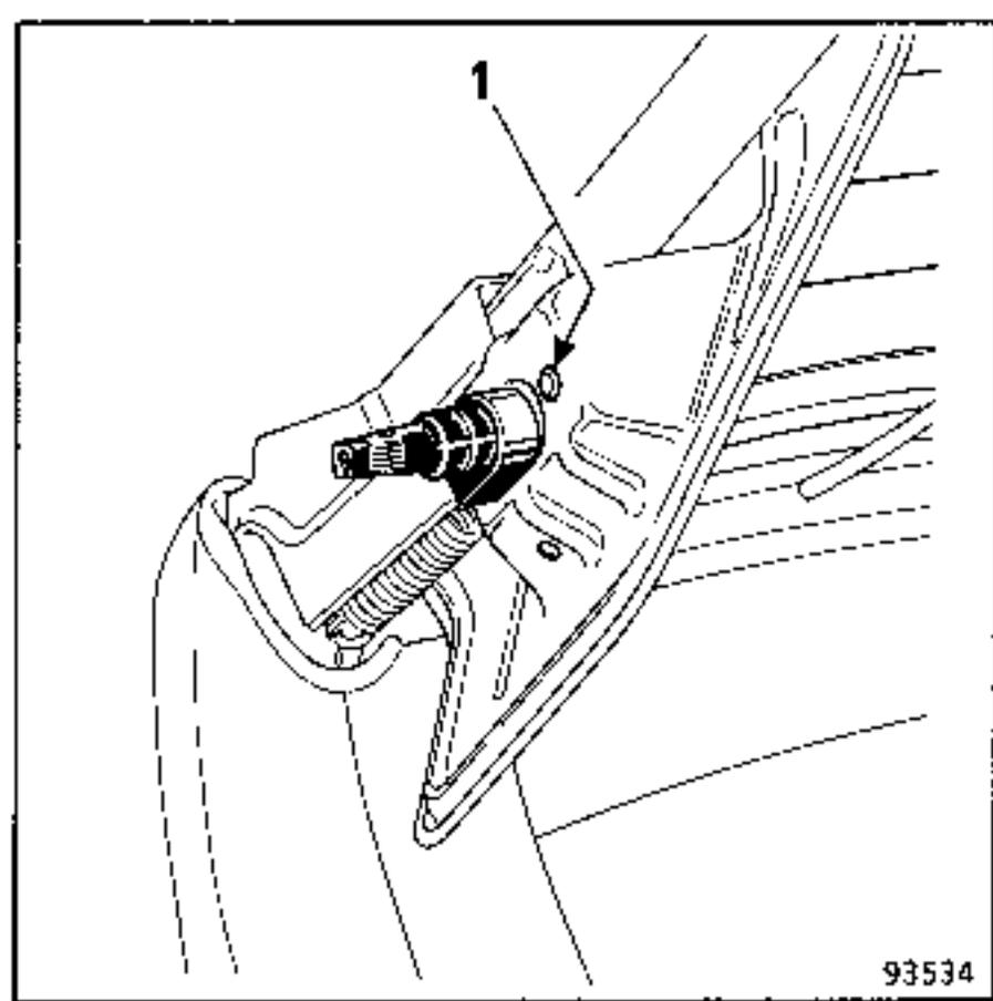
After stripping the seat back, adjust the mechanism so that it is in the slack position.
