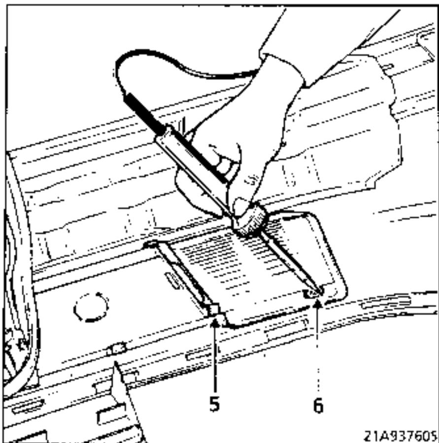
Fit the blanking cover by engaging it in the two clips (4) and on the plastic lugs (5) and (6).
