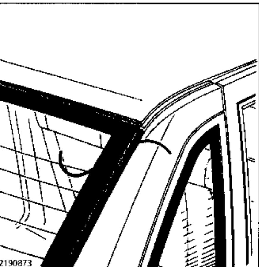
From outside the vehicle, check to see whether it is possible to pass the wire freely under the moulding mountings in all four corners of the screen when the seal is being cut. If it is not, remove the mounting or mountings which are in the way, after first protecting the frame with tape.
