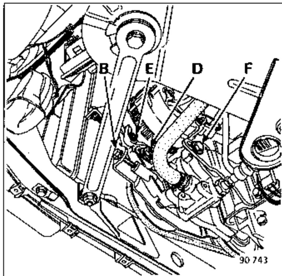
Pull the pump-support assembly to one side and secure it to the body.
