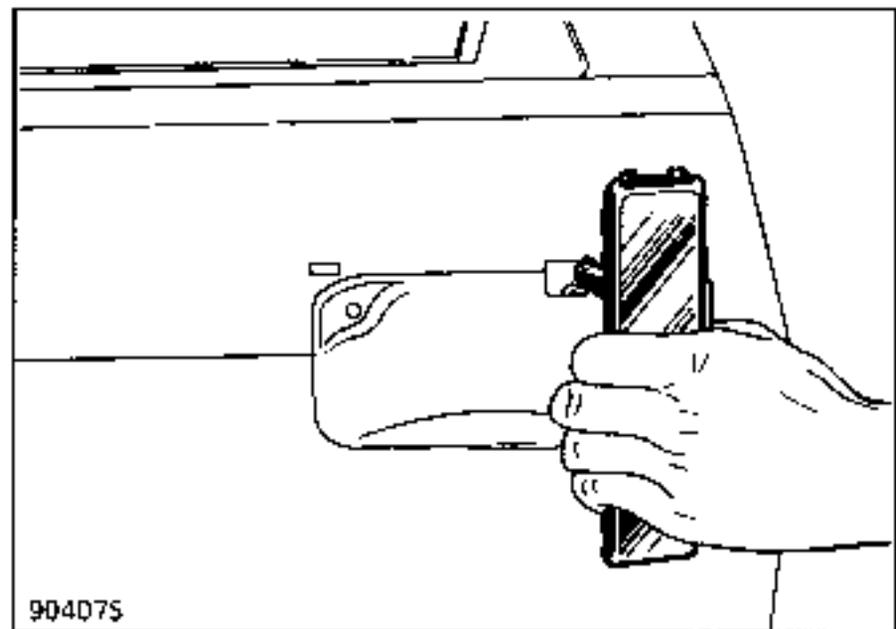
Disengage the finger plate from rod (2) holding the finger plate vertically.
