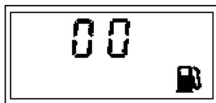
It is an indication that there is a broken circuit on the tank unit or its wiring.
