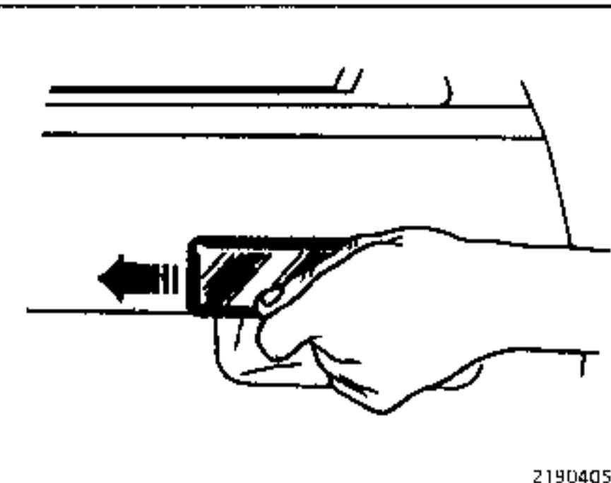
Push the finger plate forwards then disengage it from the panel.
