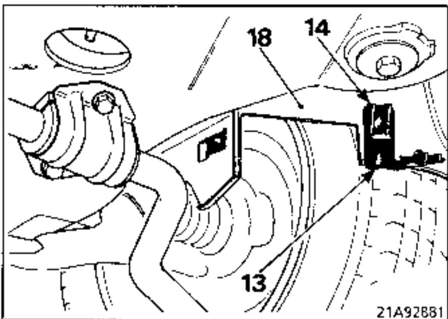
Assemble the sheet metal nuts (14) on the corner pieces (13).
