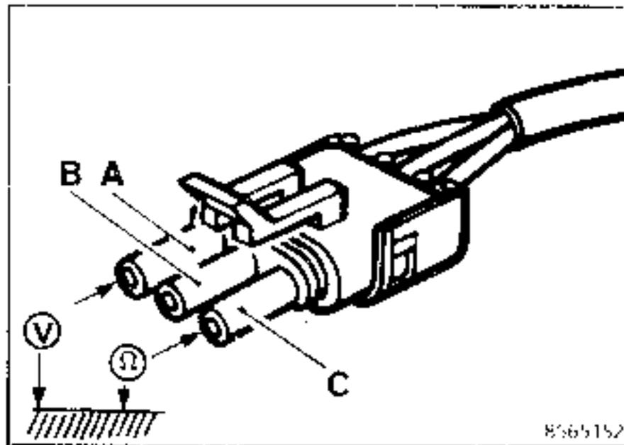
Disconnect the flow sensor and check :
