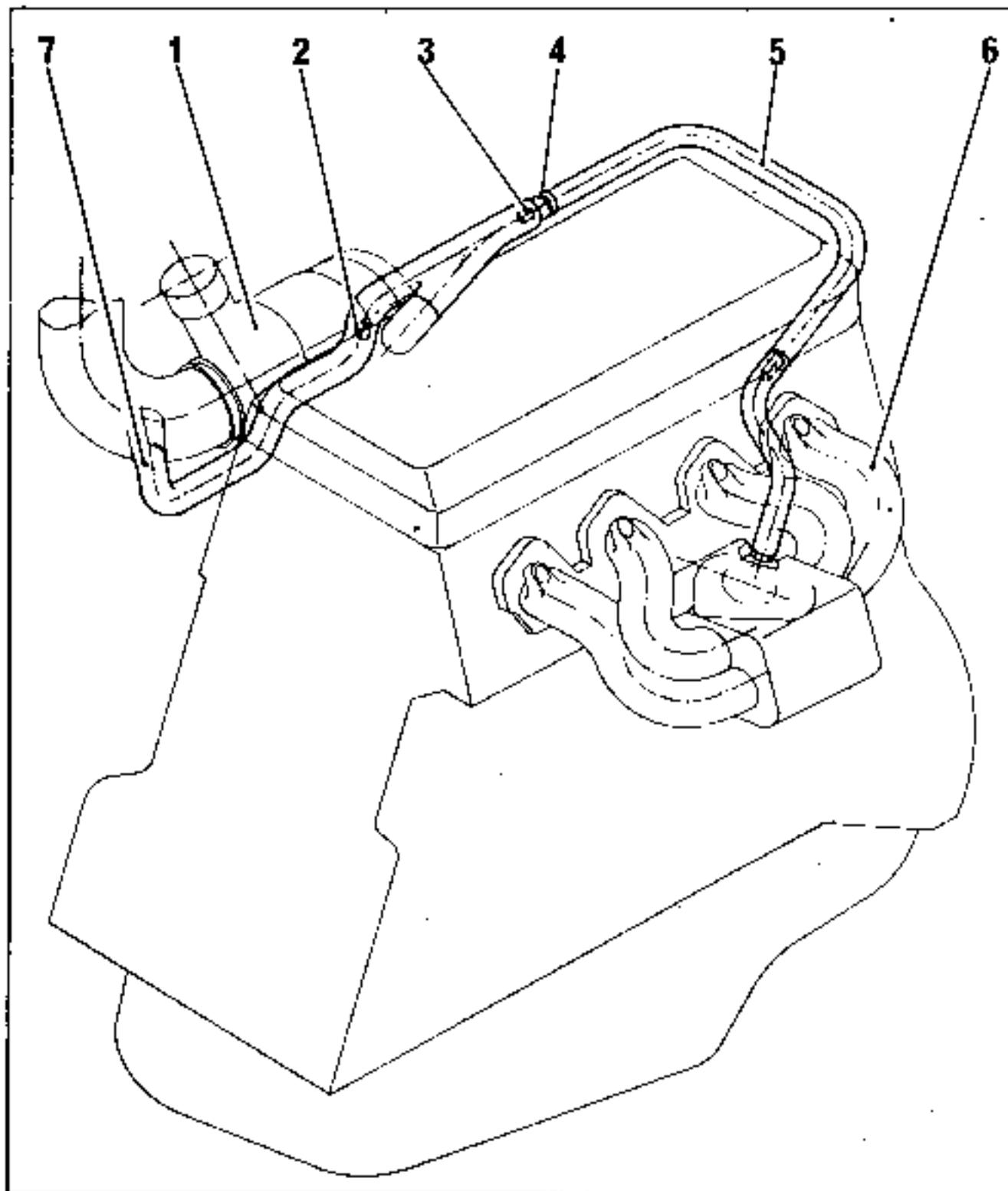
The crankcases gases are recirculated. They are taken from the rocker arm cover to the inlet manifold through a dual circuit (input and output) to be burnt in the combustion chambers. When the turbocharger is operating, valve (4) closes the output circuit.
