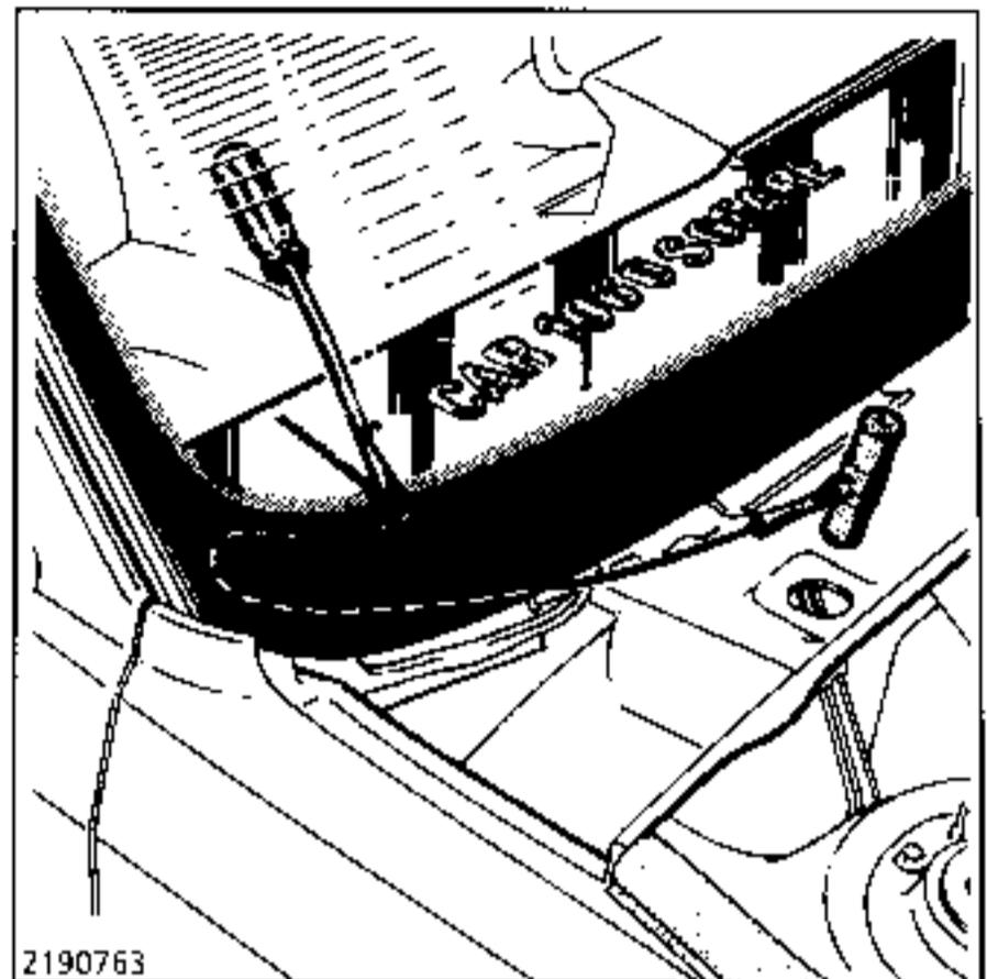
For the lower corners, pass the wire under the window and pull at the opposite corner so as not to damage the upper corner of the wing.
