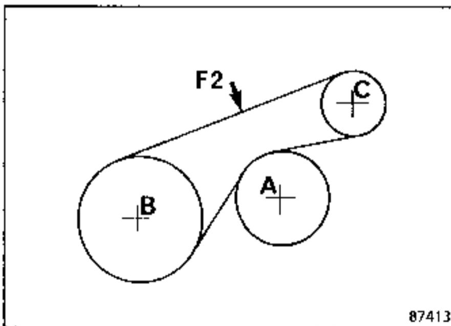
Coolant pump-alternator belt
