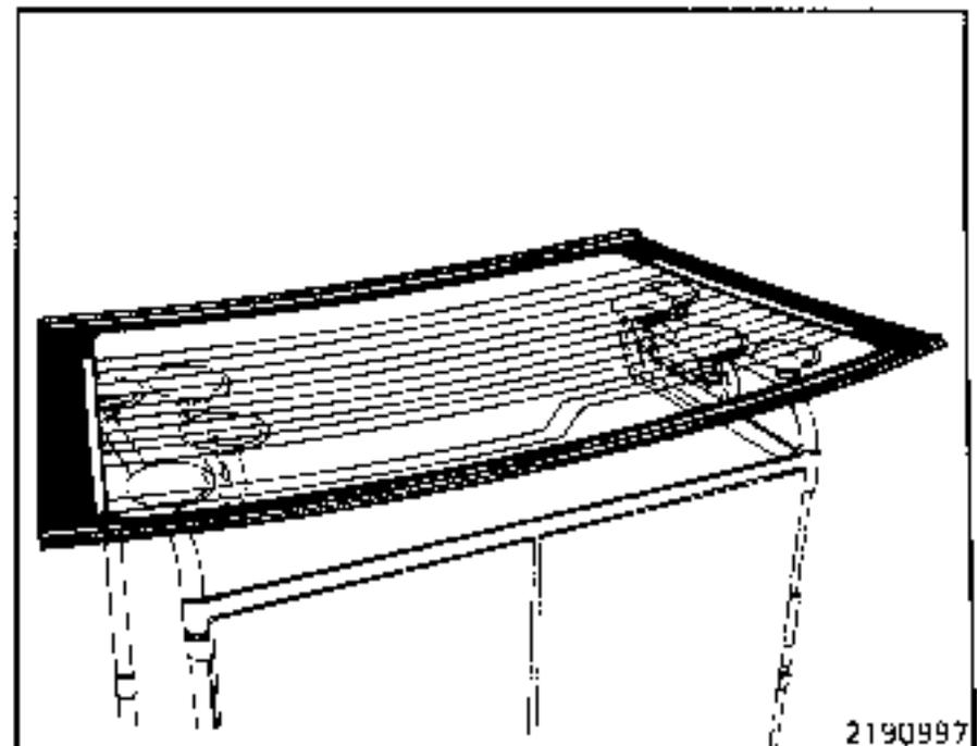
Fit the upper and lower mouldings to the edge of the screen, pushing them down to approximately half the depth of the U shape.
