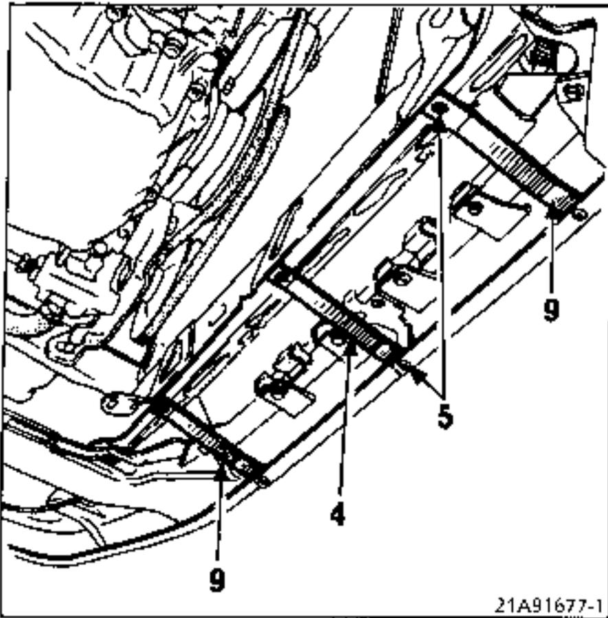
Fit the 3 connecting lugs (4) and (9) connecting the spoiler to the lower cross member by rivets (5).
