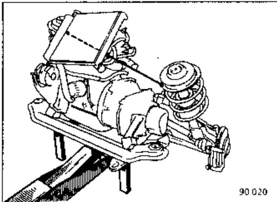
Secure the spring-shock absorber assemblies with string.
