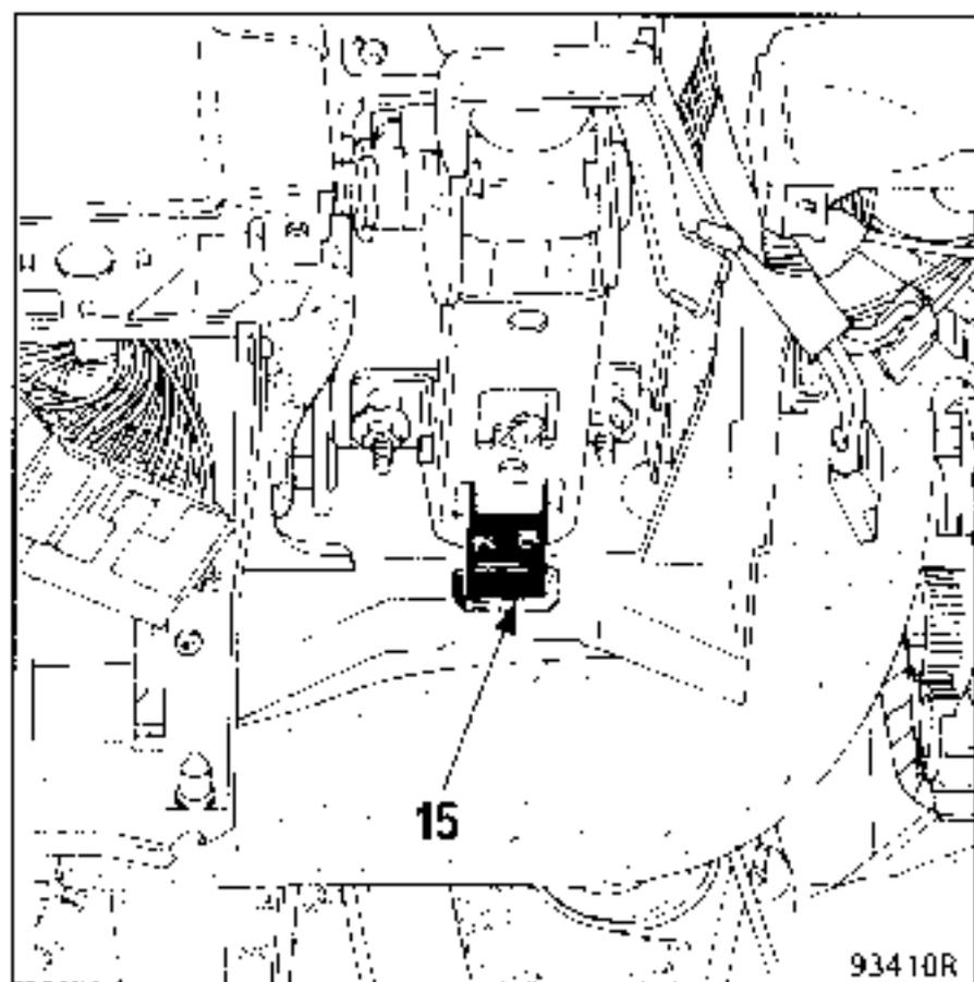
Place the steering column in position, engaging the tab (15) into its location and the steering column shaft in its universal joint.
