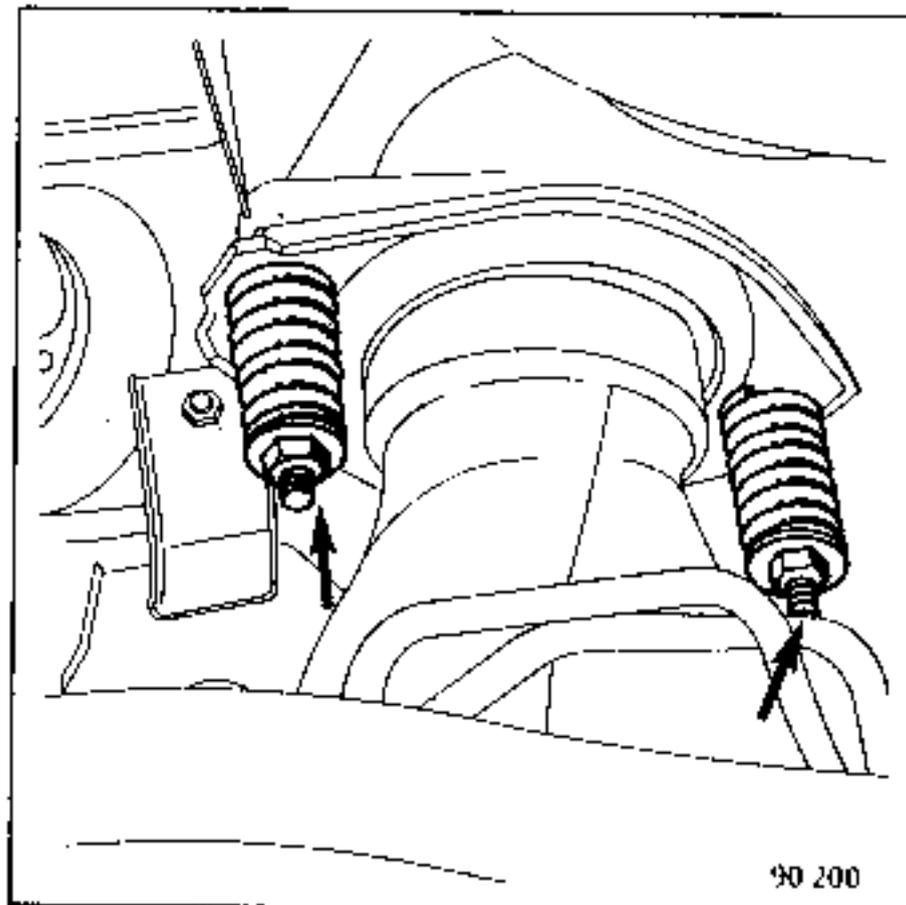
The exhaust downpipe from under the vehicle.
