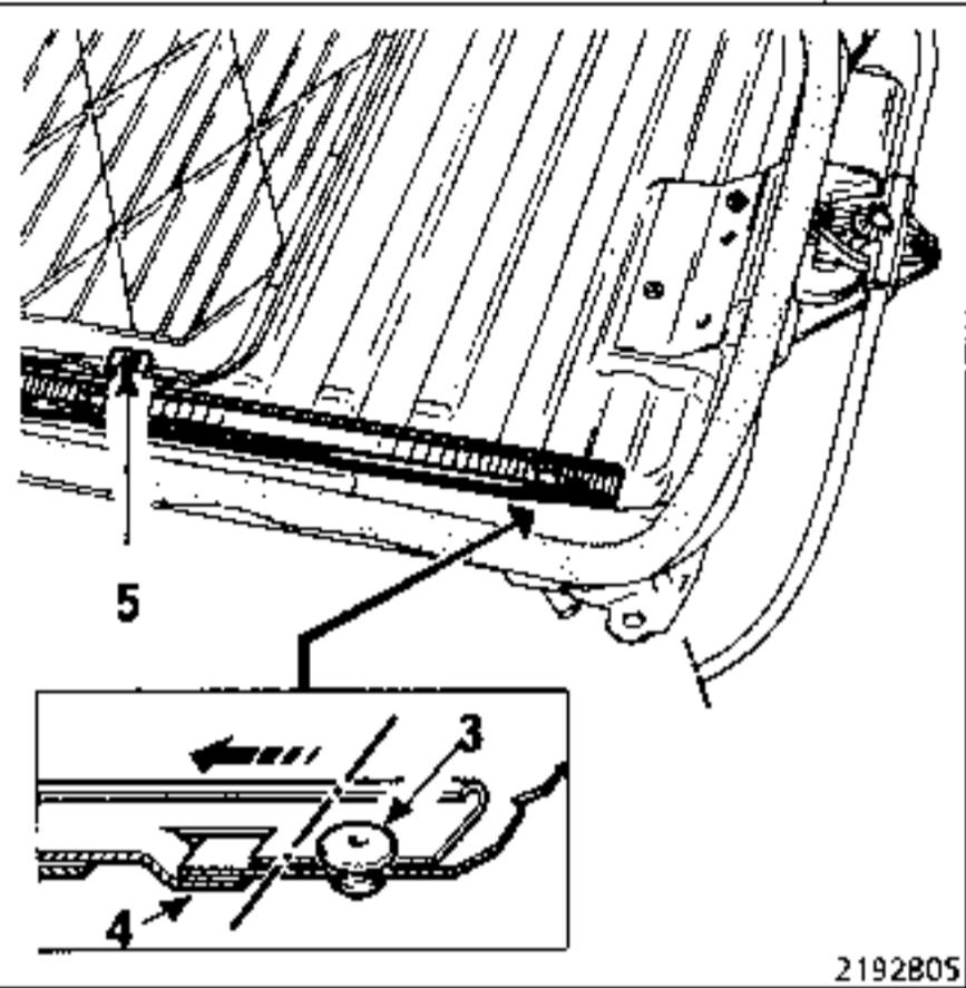
Drill the 2 rivets (3) securing the rails at the rear and remove the mechanism by pulling the rails towards the front to free catches (4).
