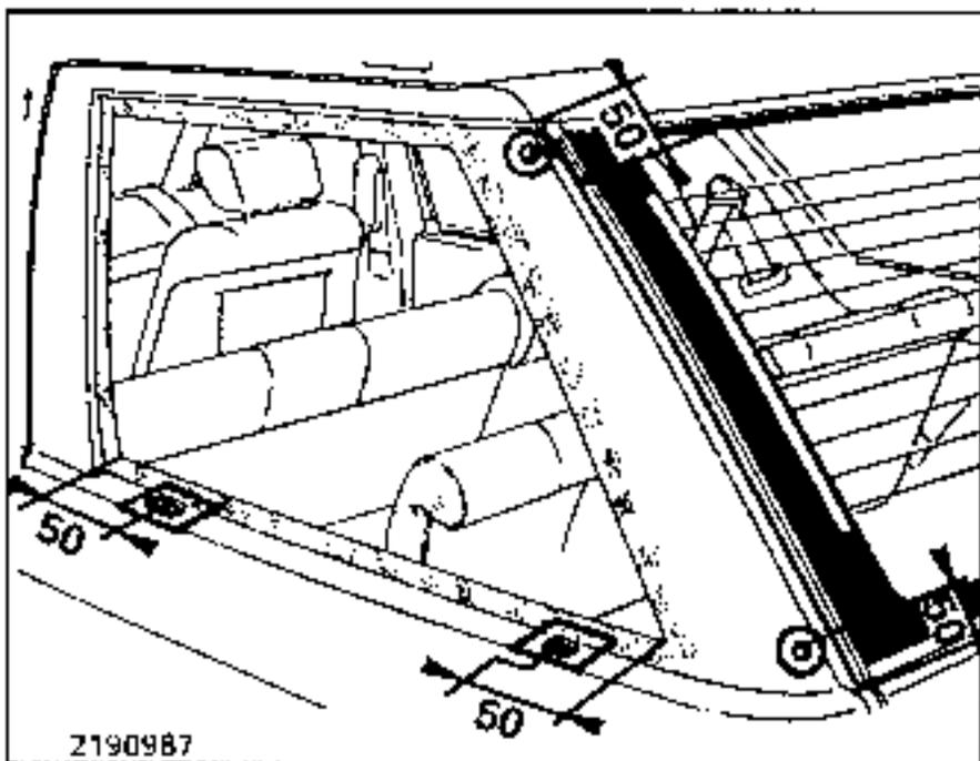
Fit the wedges for the base of the aperture and the round bearing stops as shown in the drawing above.
