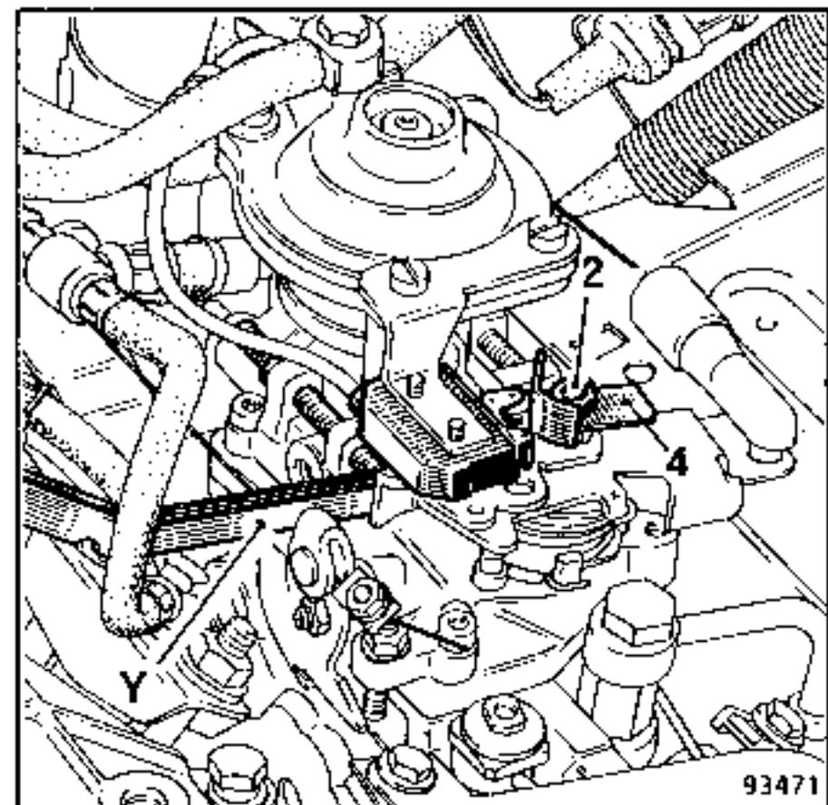
The adjustment is carried out by moving the cam on the throttle lever.
