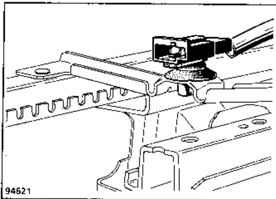
Unclip the connector from the set of slideways.
