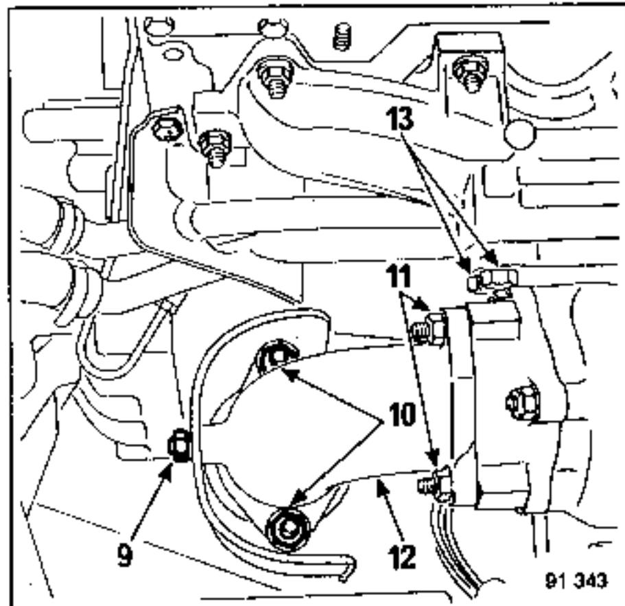
Using combination spanner FACOM No. 40, modified as shown in the illustration below, unscrew the turbocharger securing nuts (13) and remove it.
