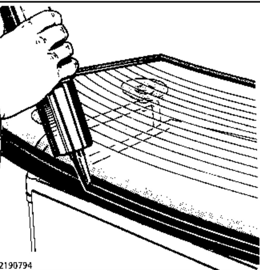
Using a spray gun apply a bead of mastic to the screen passing along the anti-overflow seal. Use a spatula to smooth down the join where the ends of the mastic bead meet.
