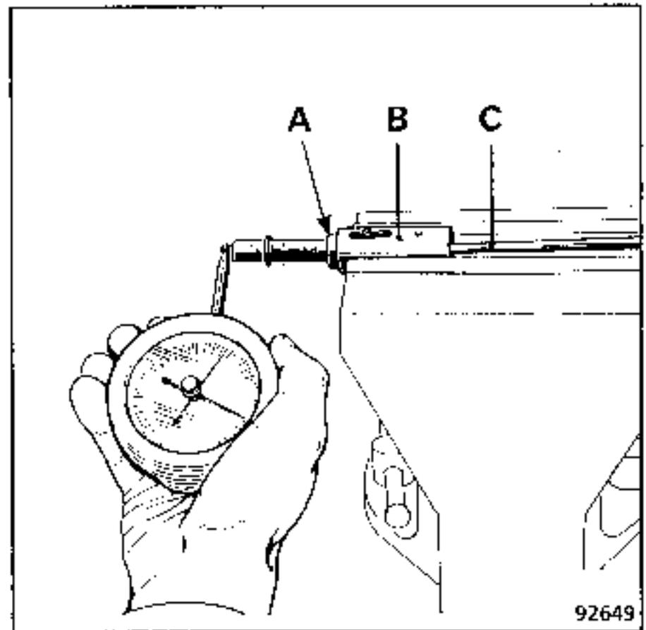
Grip tool Ele. 346 in a vice after first removing its plug. Apply the cylindrical part of tool B.Vi.906 to the end of the sliding part. The shoulder (A) should be flush with the plunger body (B) when the pointer shows 3 daN. If it is not, adjust screw (C) to increase or reduce the spring pressure.
