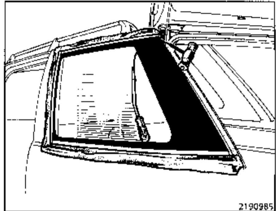
Cut the mastic bead as shown in the drawing above.
