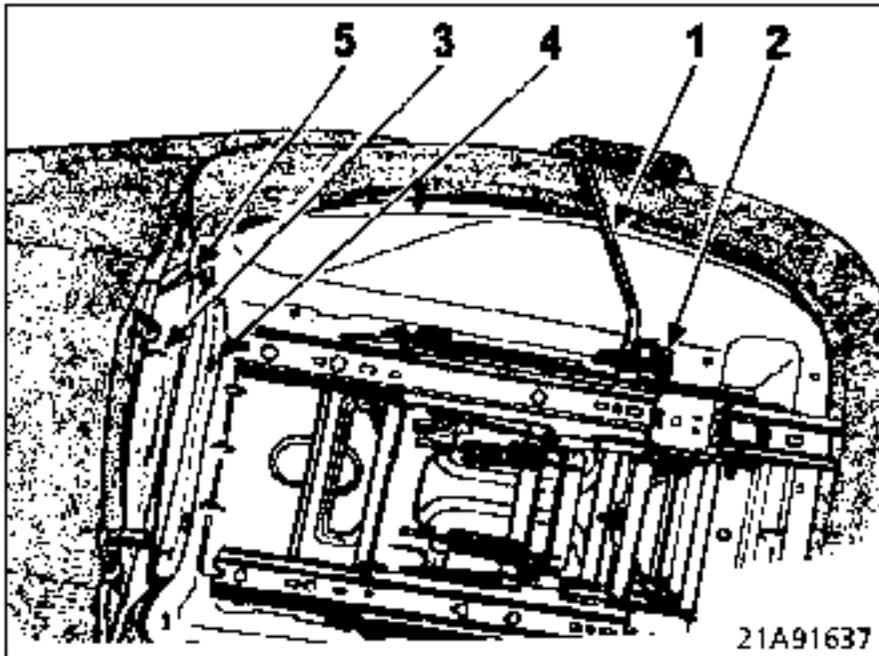
Cut clips (6) securing the three trim rods to the foam.
