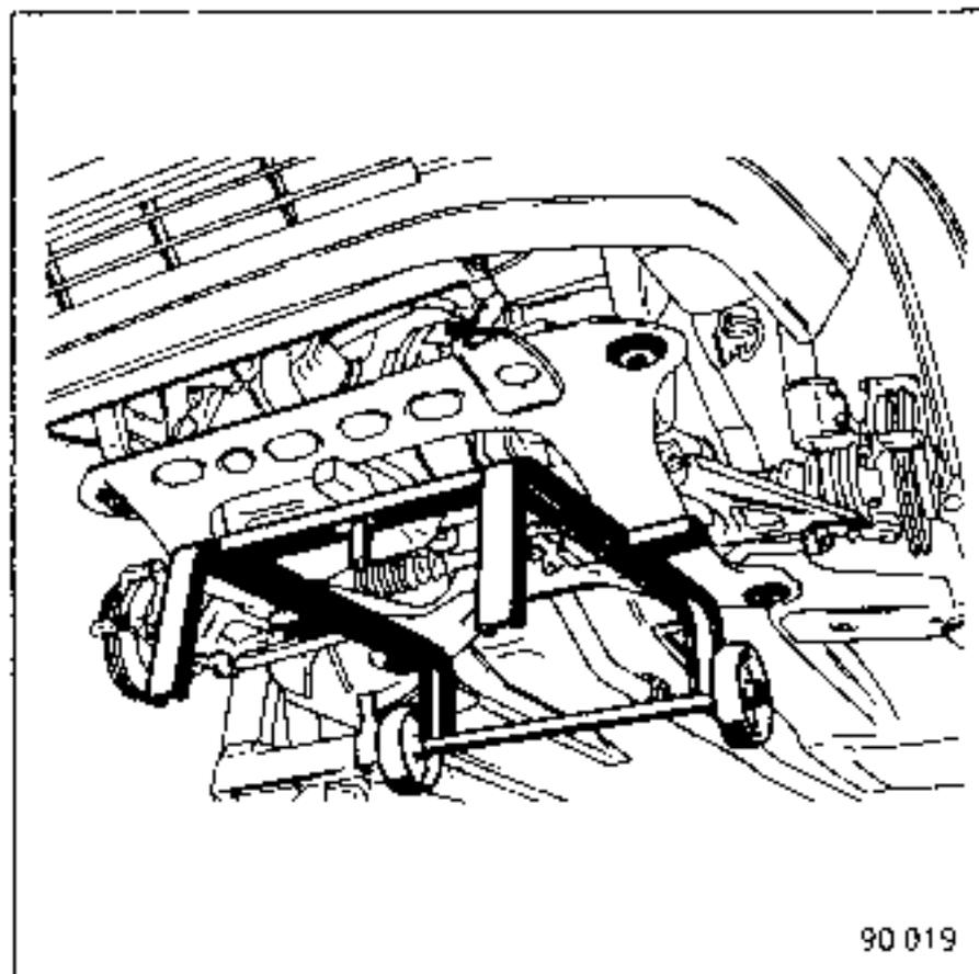
Lower the lift until the dummy sub-frame makes contact with the floor.
