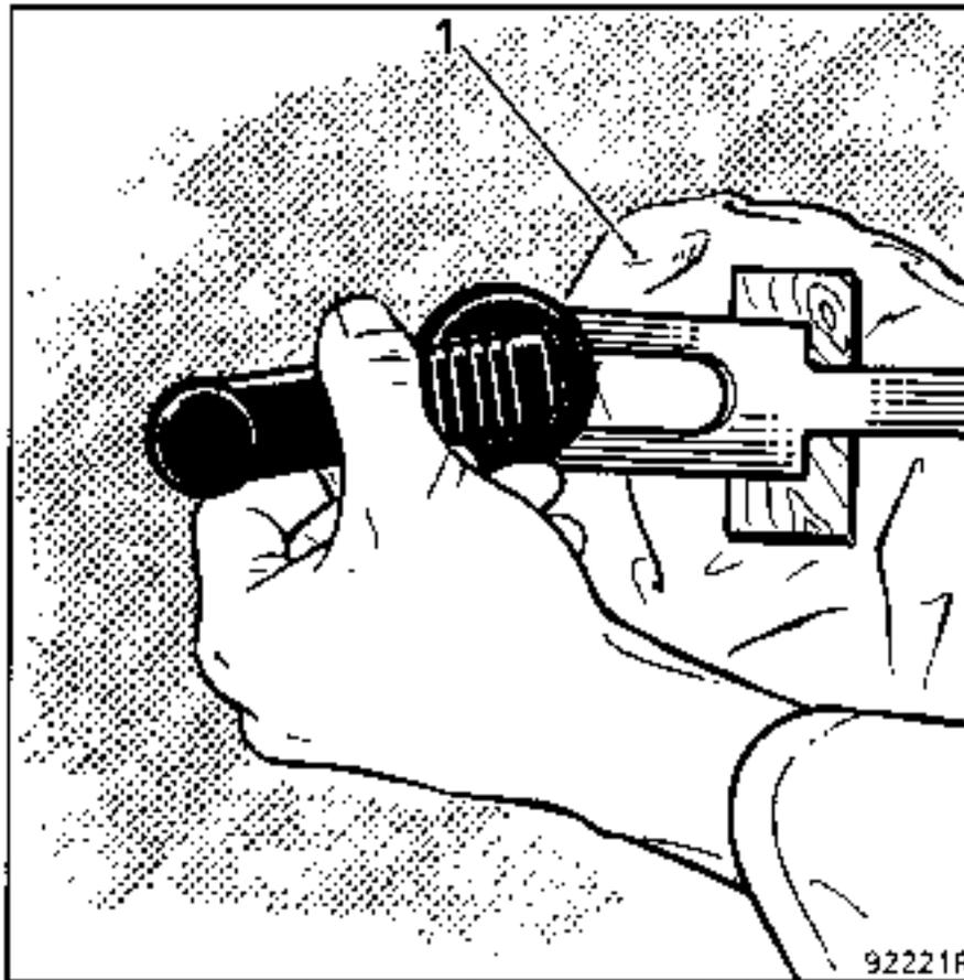
Use a locally made up fork or tool **FACOM D115** as a lever to remove the window winder, taking care to protect the door trim with a piece of cloth (1) and to place a block between the cloth and the tool.
