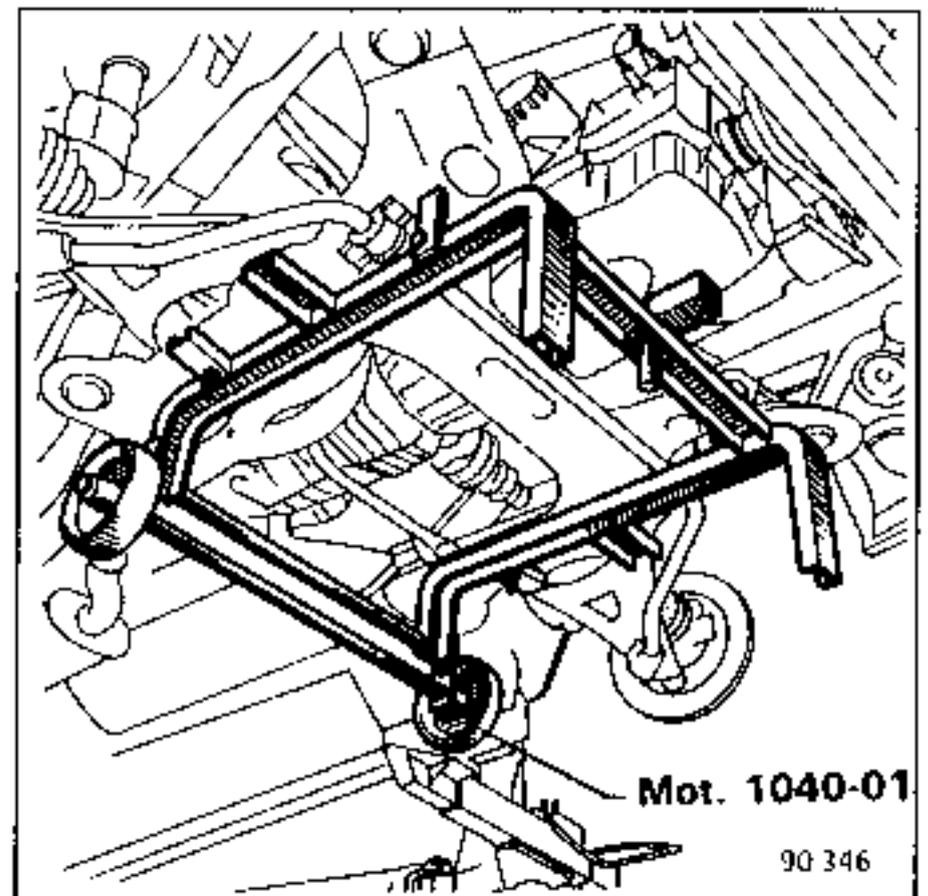
Lower the vehicle, fitted with sub-frame
