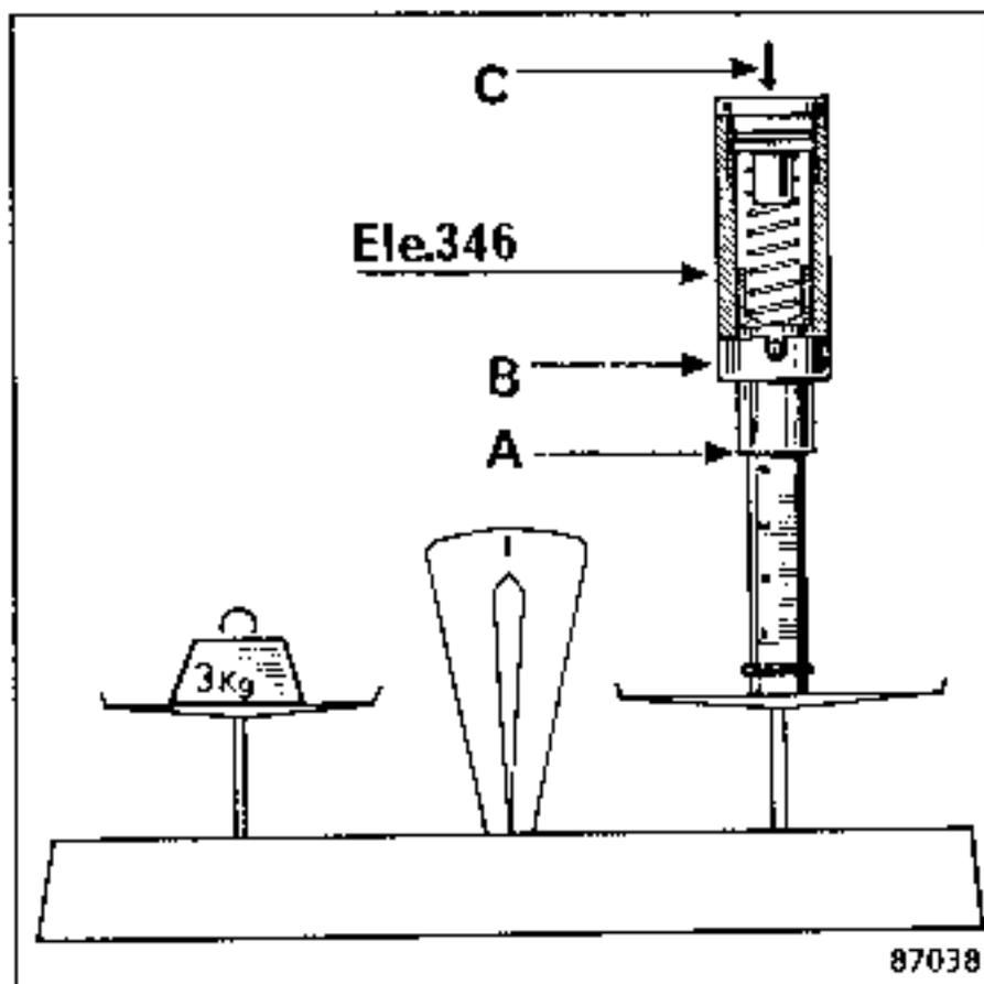
Apply a force of 3 daN (weight of 3 kg) to the tool. The shoulder (A) should be flush with the plunger body (B). If it is not, turn the screw (C) to increase or reduce the spring pressure.
