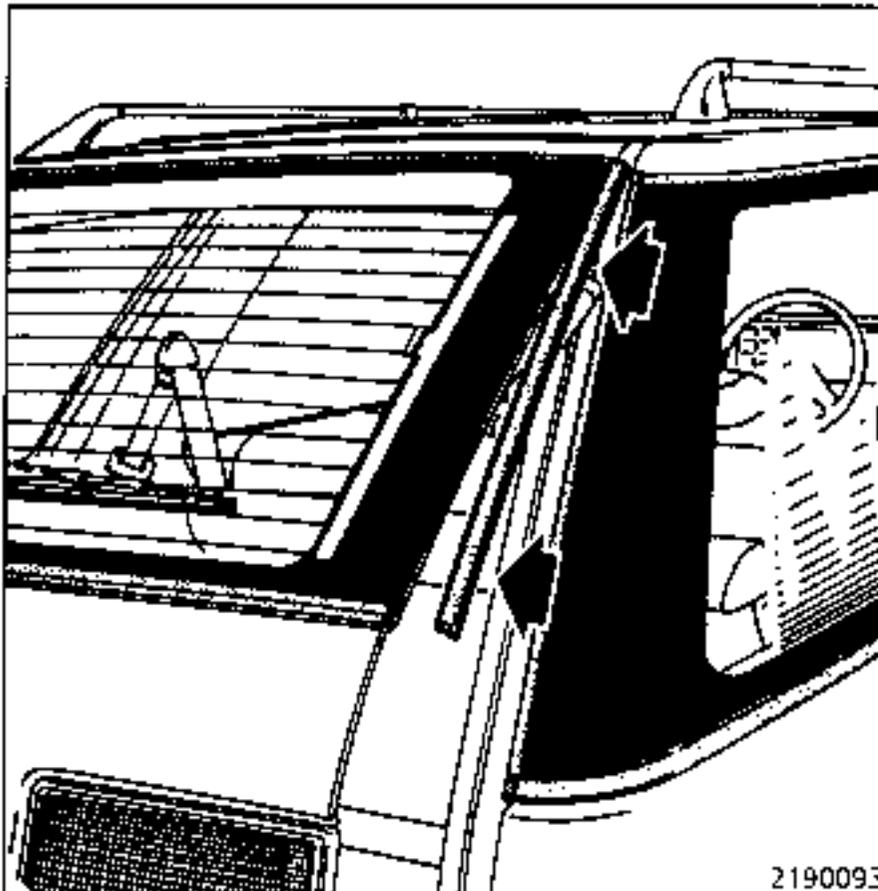
Fit the side trim pieces to the screen and adjust the position of the screen to bring it in line with the quarter lights..
