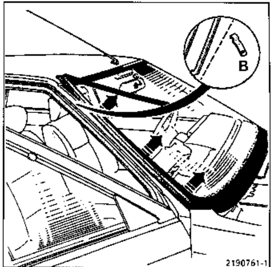
Use the remaining mastic to apply a thin bead to the area of the aperture or in the groove of the new moulding.
