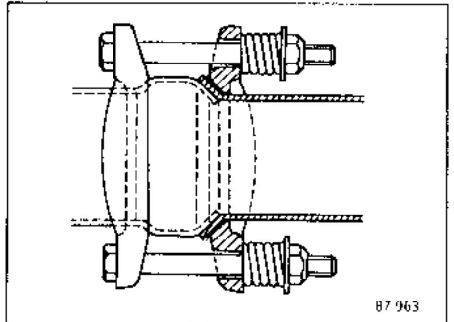
The spherical joint is sufficiently tight as soon as an effective seal between the 2 pipes is obtained.
