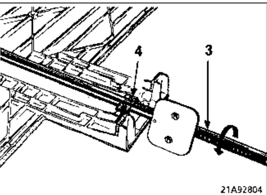
Turn the guide tube (3) on its shaft, around hook (4), to separate it from the screen.
