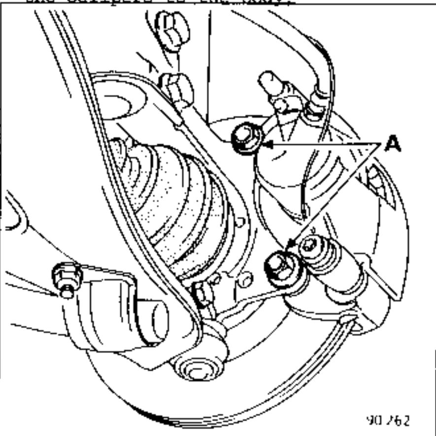
Disconnect the steering ball joints using tool T.Av.476.
