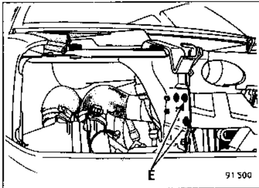
REMOVING the adjacent components
