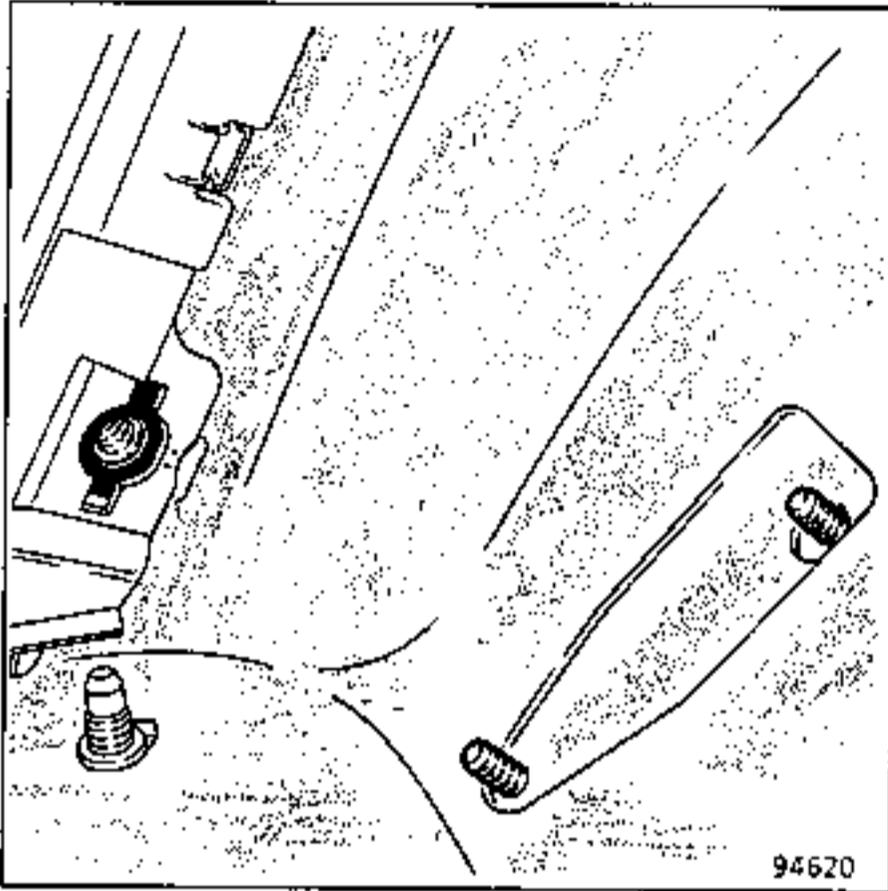
Remove the lower mounting bolt from the bodywork.
