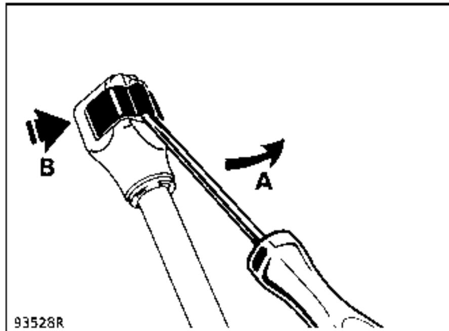
To remove the strut, using a screwdriver move aside the metal clip (A) - but do not remove it - and take the pivot pin out of its location.
