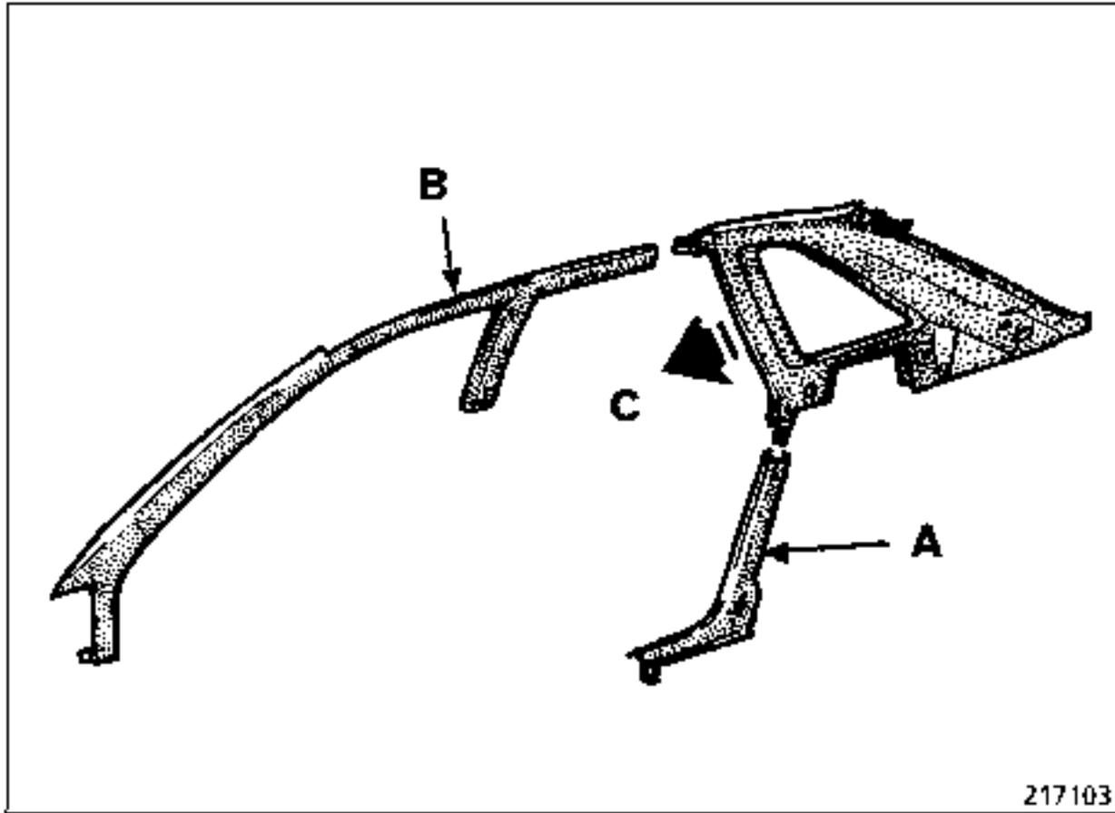
In order to remove the rear quarter panel trim, the rear pillar trim (A) must be removed as well as part of the body side upper trim (B). When the securing screws have been removed, free the trim by moving it towards the front of the vehicle (C).
