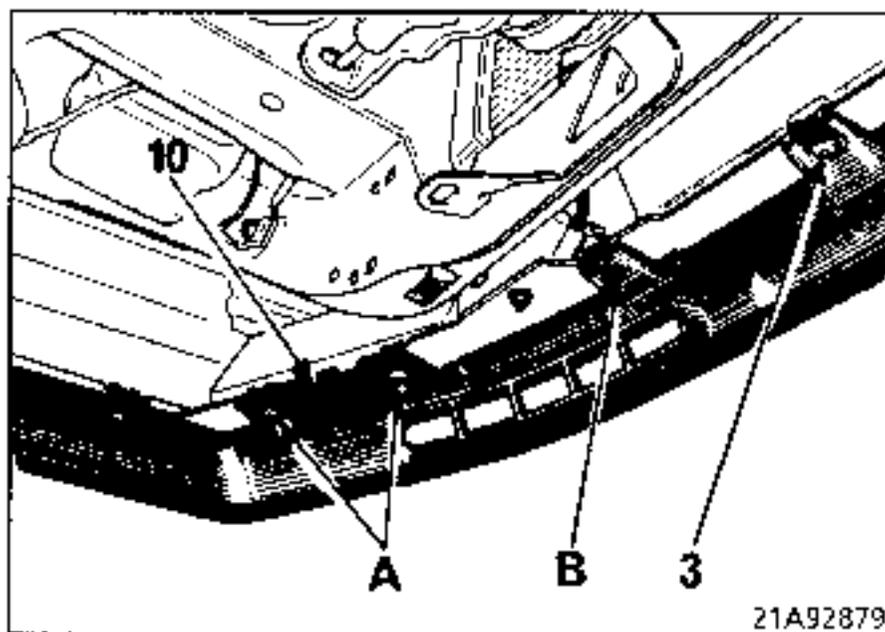
Fit the spoiler to the vehicle and secure it using the captive washer bolt (3).
