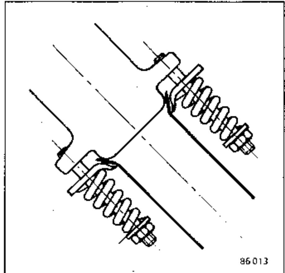
Fit clamps Mot.453-01 to the heating
