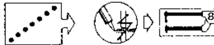
(A) 1 spot weld joining 3 thicknesses
