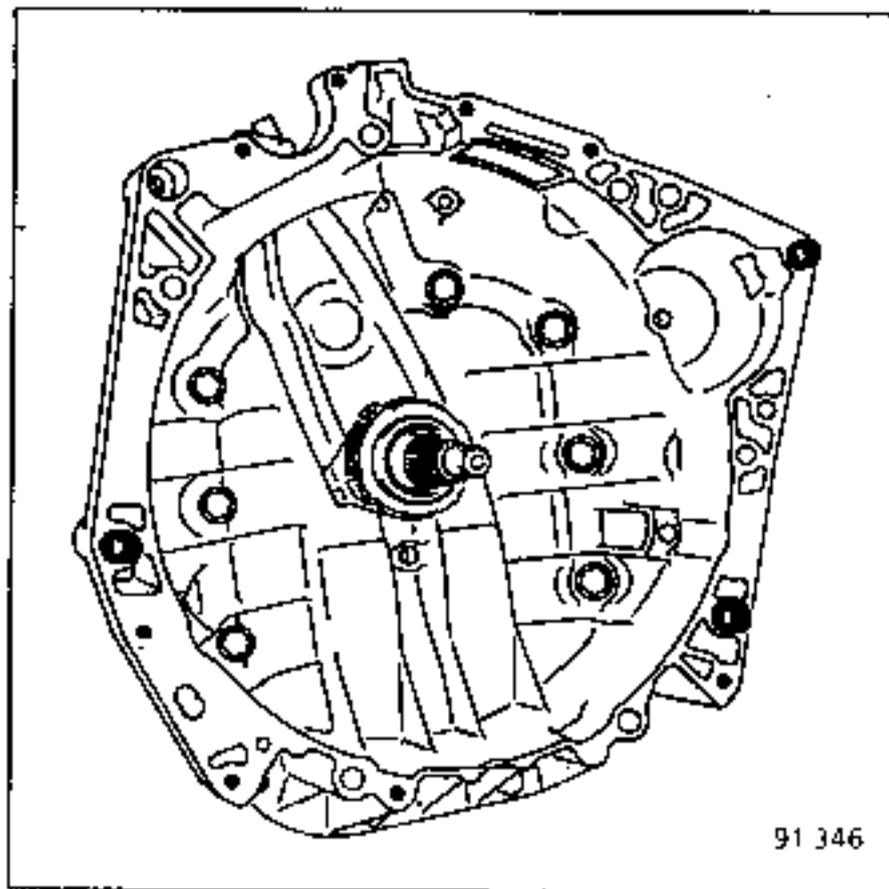
Grease the splines on the primary shaft with no. 20 grease.
