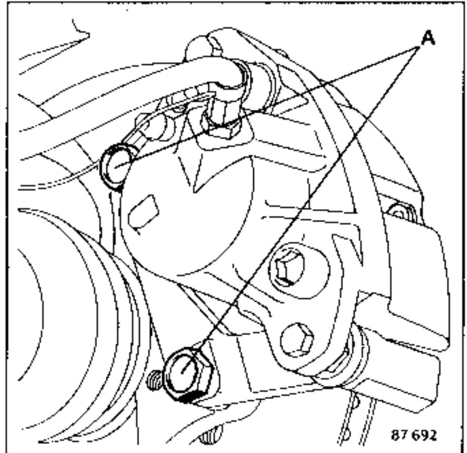
Loosen the sub-frame securing bolts.
