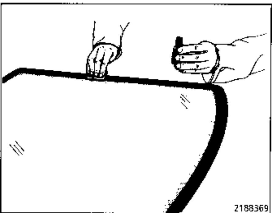
2) Then, use a degreasing solvent, using the special cloth supplied in the kit.
