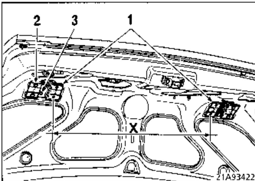
Fit in place the two strengtheners (1) using screws (2), but do not tighten them. Centre them and adjust the distance X between them to the dimension shown in the drawing :
