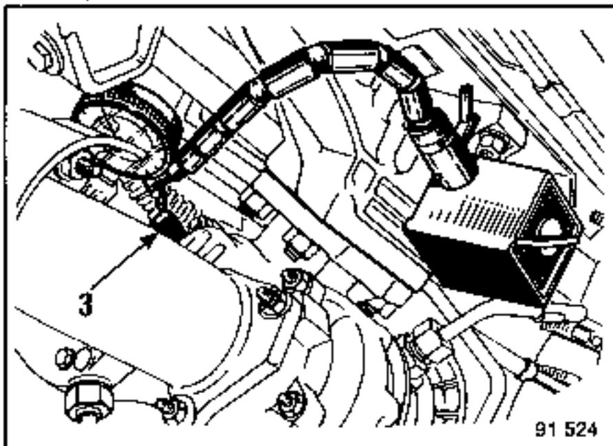
Slowly increase the pressure until the adjusting rod has moved by  $0.38 \pm 0.02$ mm and note the pressure gauge reading which should be within the checking values stated.
