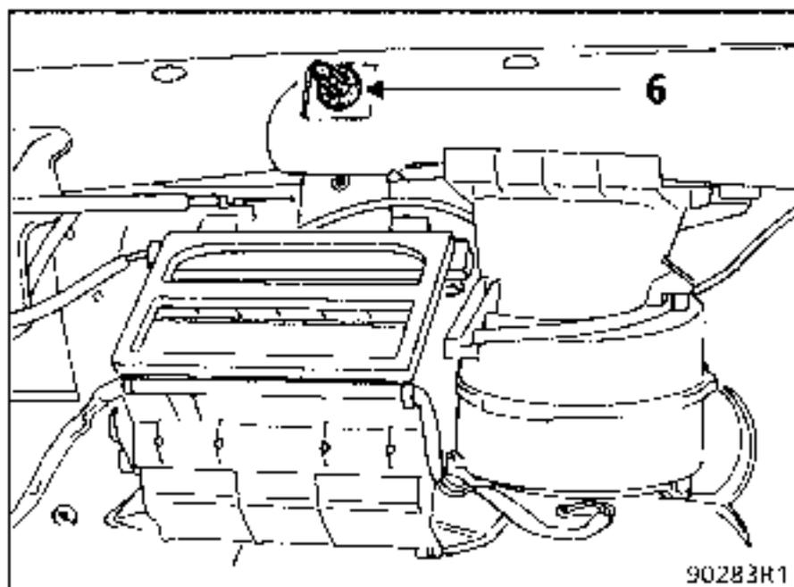
Place the fascia panel in position and fit it on to the locator (6) (take care not to trap the wiring) and secure the fascia panel in place.
