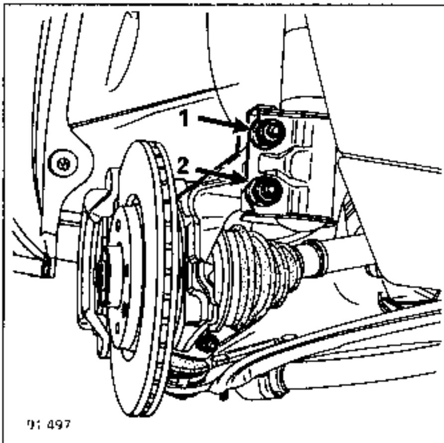
Tilt the stub axle carriers and disconnect the drive shafts.
