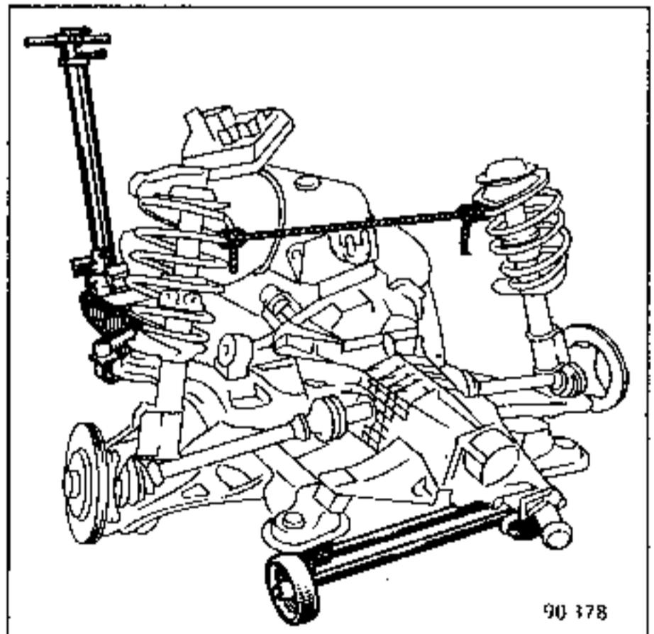
Secure the spring-shock absorber assemblies with string.
