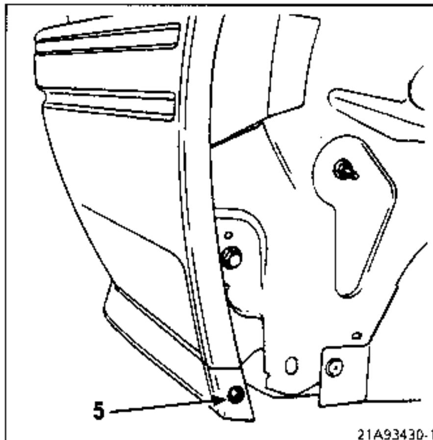
Secure the spoiler at the ends using the two screws (5).
