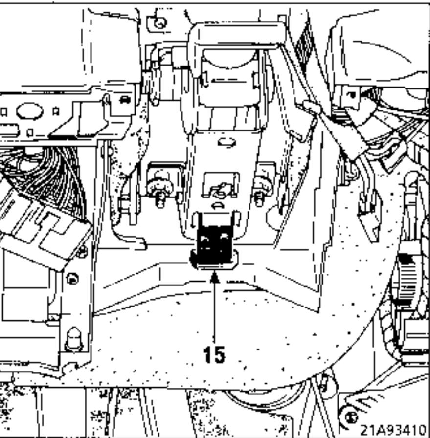
Offer up the steering column, engaging tab (15) in its location and the steering shaft in the universal joint.
