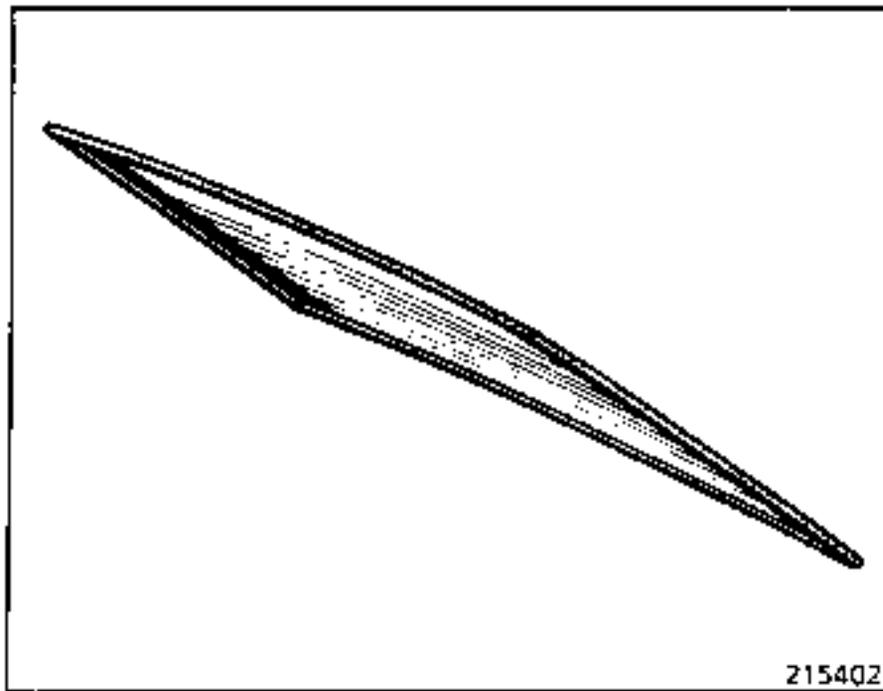
This window is of the moulded type, that is, the moulding is moulded around its edge. It is impossible to separate the moulding from the window.
