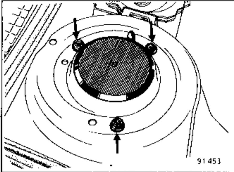
Remove the sub-frame securing bolts.
