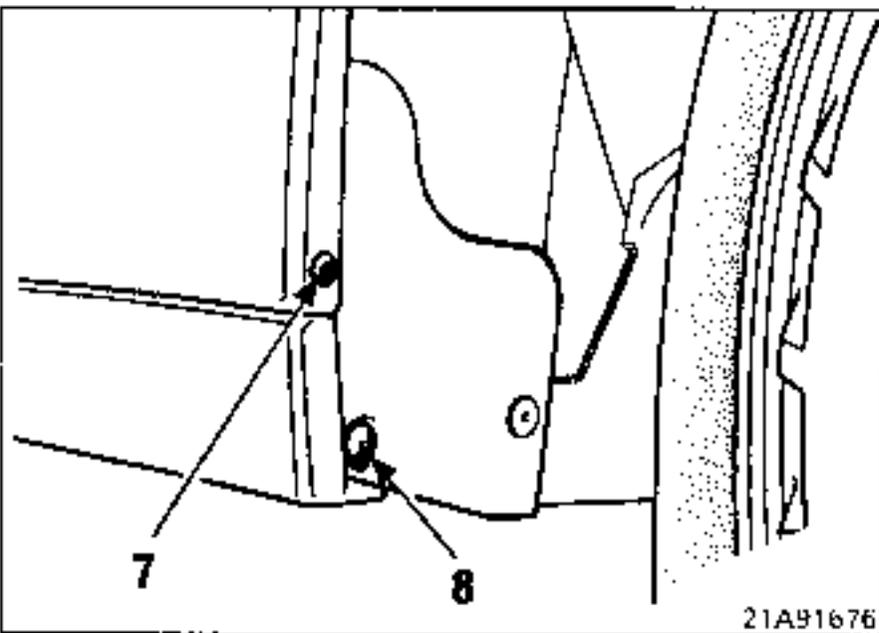
Secure the ends of the spoiler using sheet metal screws (7) and rivets (8).
