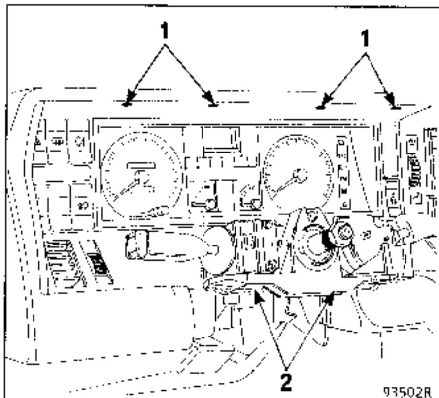
Disconnect the speedometer drive cable.
