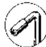
(A) 1 spot weld joining 3 thicknesses
