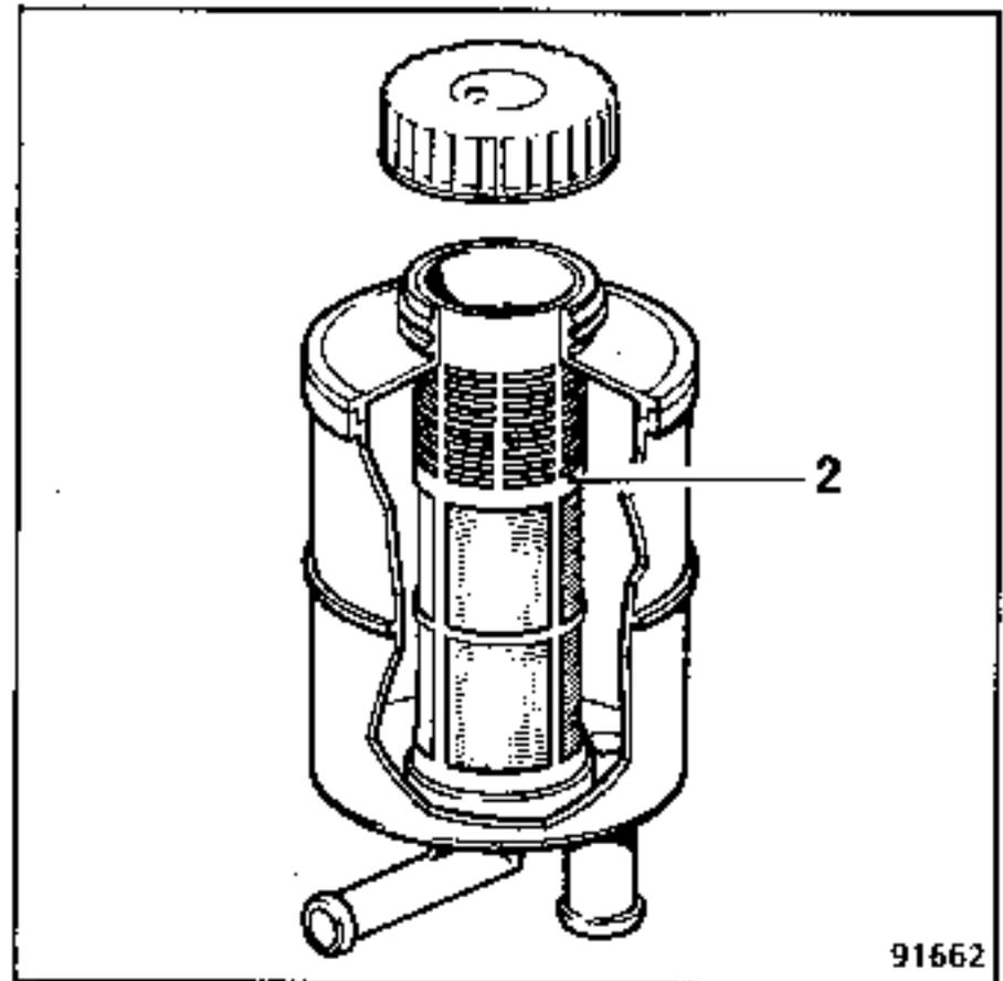
The oil should come up to the band (2) on the filter sleeve.
