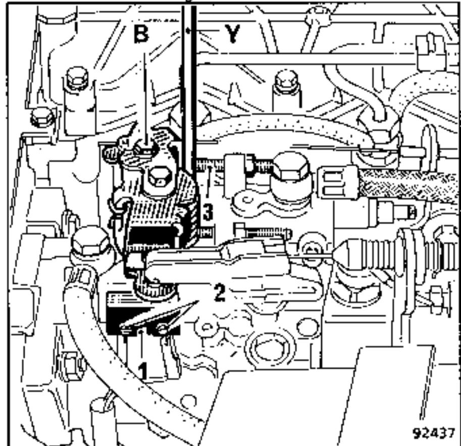
The system is adjusted by moving the micro switch (1) on its support.
