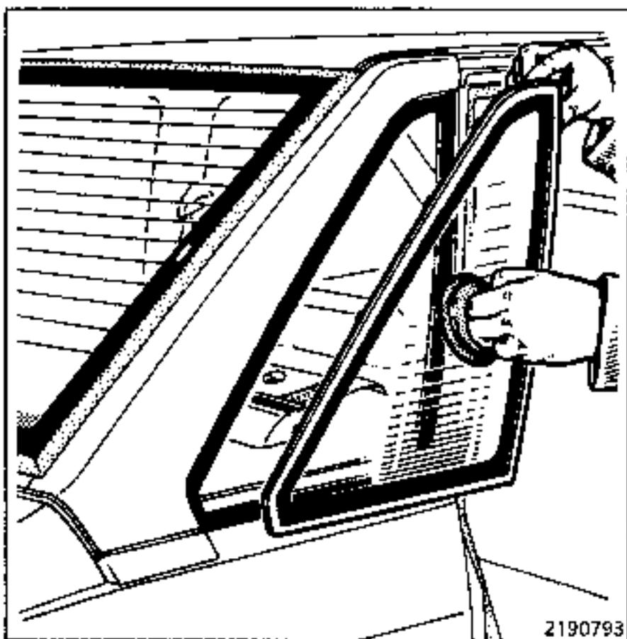
Using a single suction pad (for the part number see the beginning of the section), fit the window to the vehicle offering it up parallel to the aperture.
