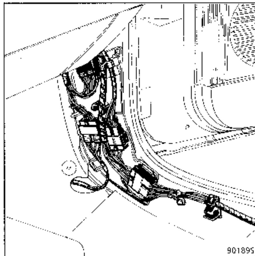
Do not forget to reconnect the connector (5) on the fascia panel harness, the windscreen wiper harness and the pedal assembly connector.
