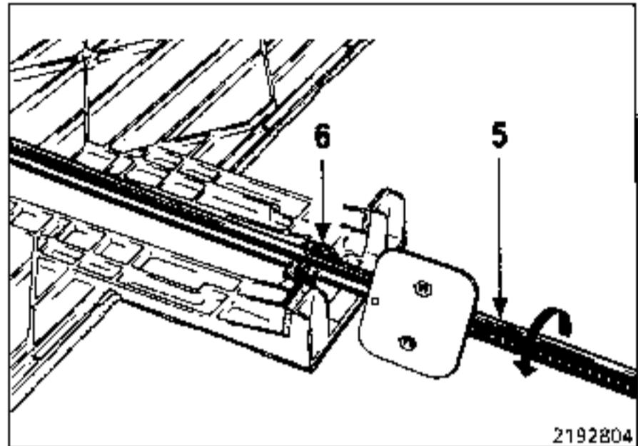
Pivot the guide tube (5) on its shaft around hook (6) to separate it from the screen.
