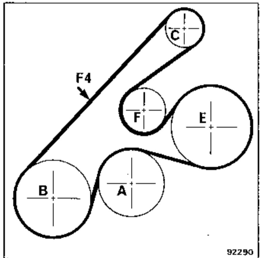
Coolant pump-compressor-alternator belt
