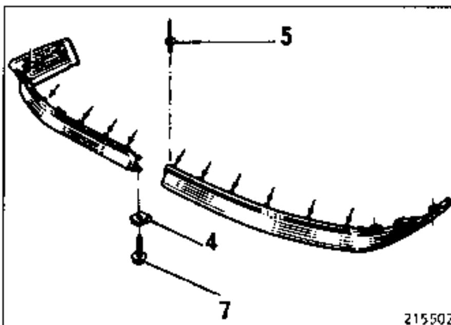
Fit the spoiler to the shield (in the order given above) and secure it using bolts (3), (8) and (7), after first positioning the sheet metal nuts.
