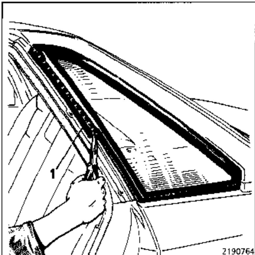
**NOTE :** Removal of the window means that the moulding frame must be replaced.
