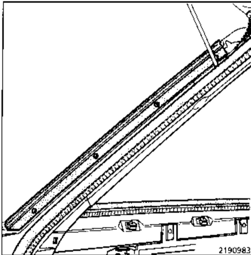
Remove the 4 rivets holding the rear moulding.
