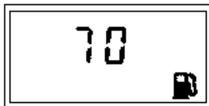
It is an indication that there is a short-circuit on the tank unit or its wiring.
