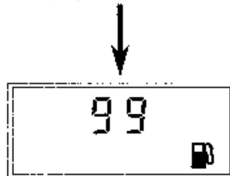
It is an indication of a broken circuit on the tank unit or its wiring.
