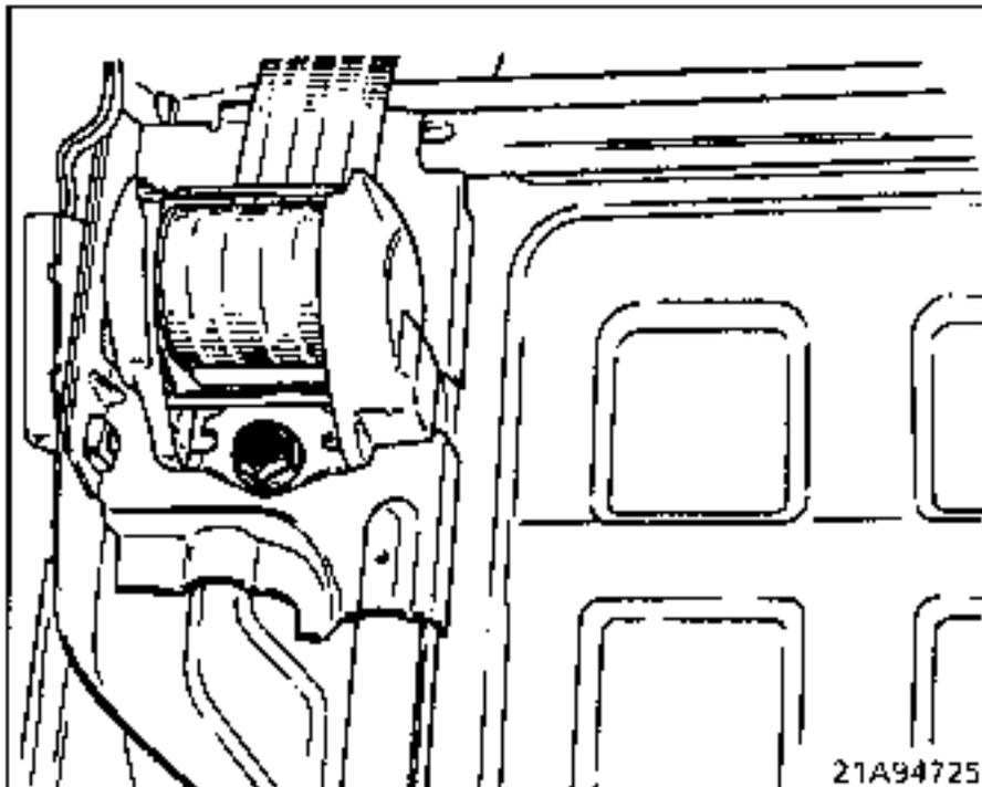
After removing the seat back trim, remove the seat belt mounting.
