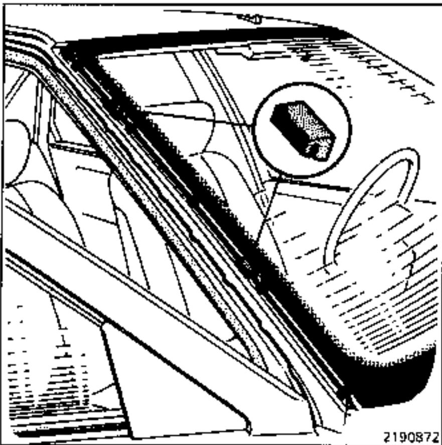
To make it easier to centre the windscreen at the sides, fit the Renault 25 locating wedges to be found in the bonding kit, to the windscreen aperture.
