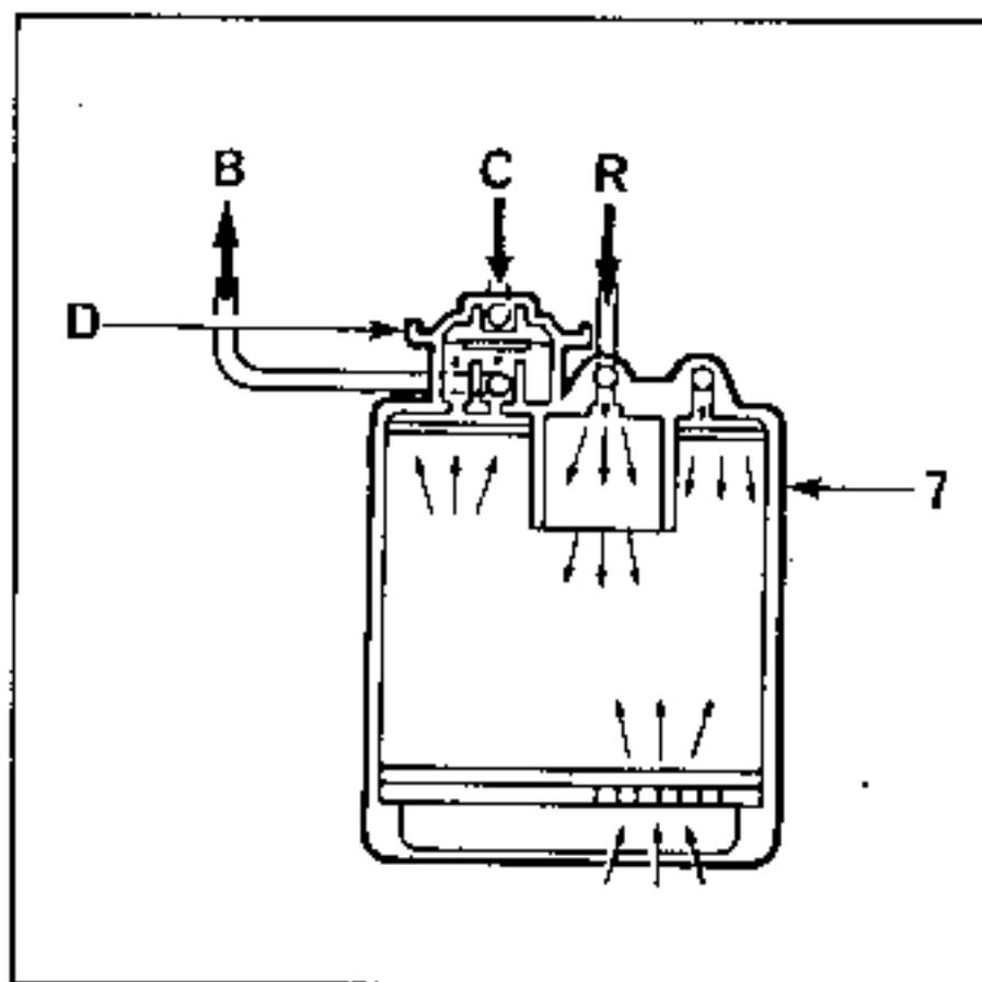
For certain markets, X 48K vehicles are fitted with a system for absorbing the vapours emanating from the fuel tank:
