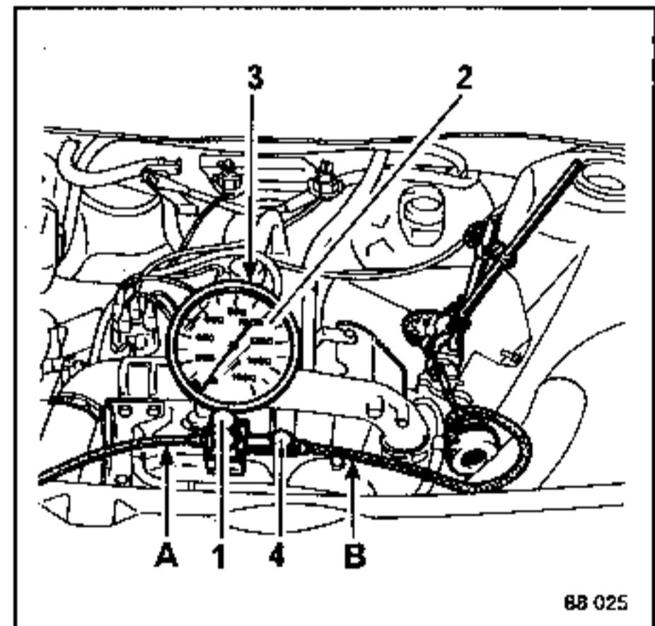
Before using the equipment, zero the pressure gauge (screw 3), fully unscrew the pressure reducing valve screw (1) and the leak screw (4) and connect the inlet pipe (A) to the compressed air supply.
