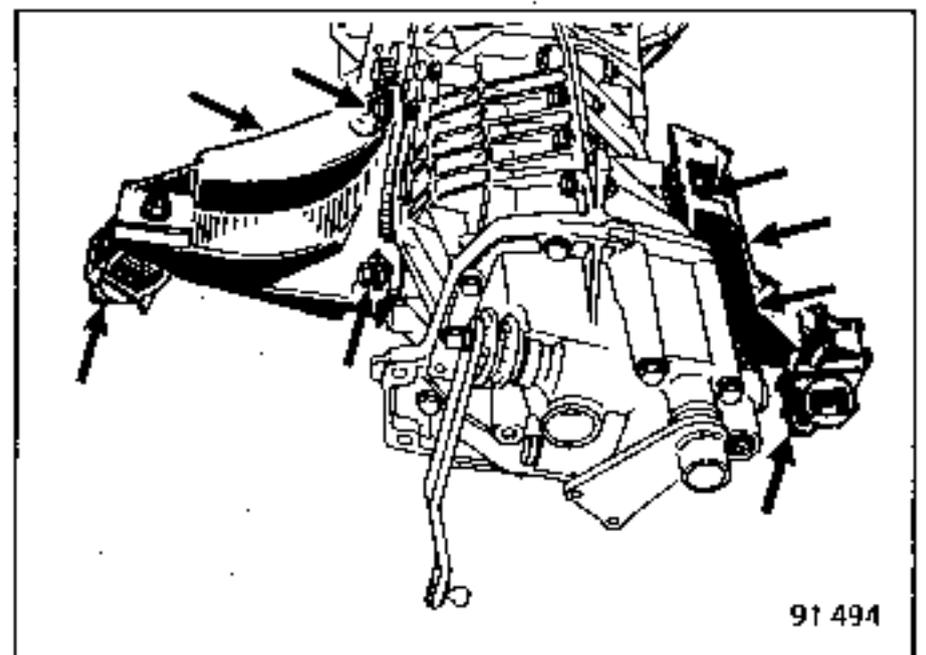
Secure the computer unit and the power steering reservoir to the engine.
