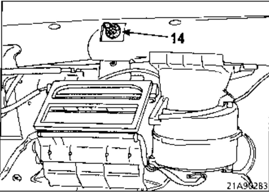
Check that the plastic locating device (14) is fitted.
