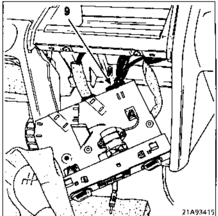
Disconnect the electric feed connector (9) (colour brown) from the dashboard without removing it.
