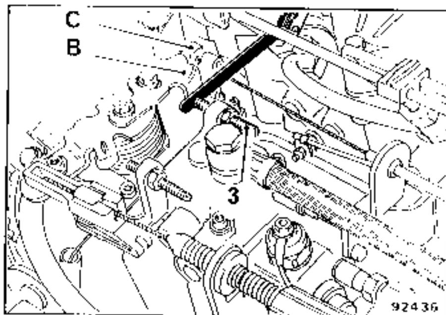
Check the initial idling speeds, with and without the 1mm feeler gauge, and if the speeds have altered, repeat the adjustments (b, c and d).
