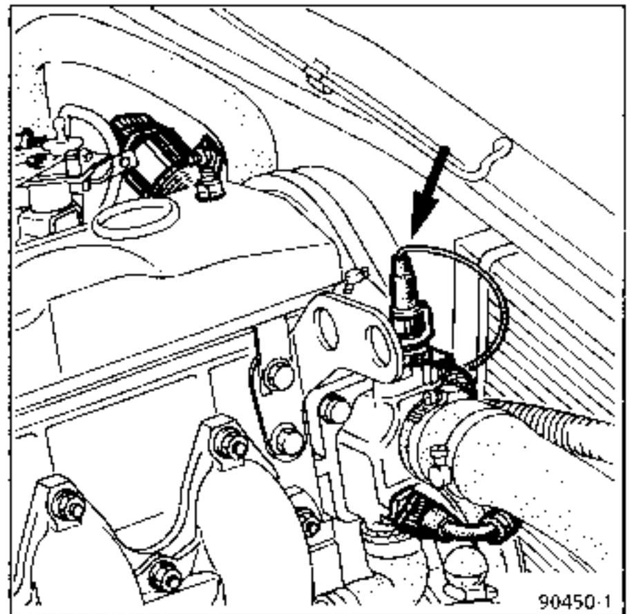
Check that the sensor is correctly connected and the condition of the terminals and wires.
