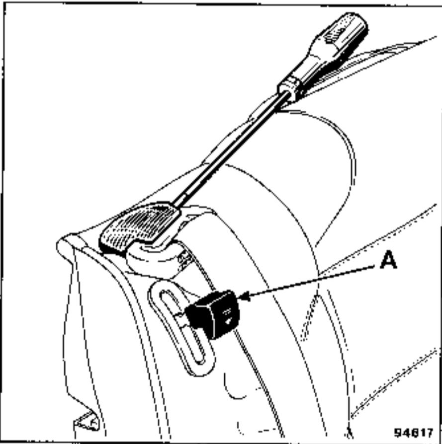
After removing the seat, remove handle (A).
