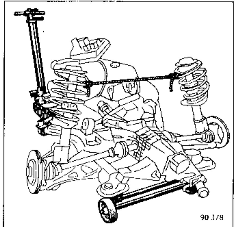
Secure the spring-shock absorber assemblies with string.
