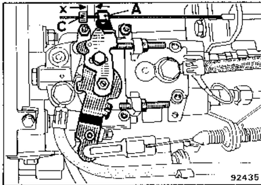
This operation must be carried out when the engine is warm after having adjusted the idling and fast idling speeds.
