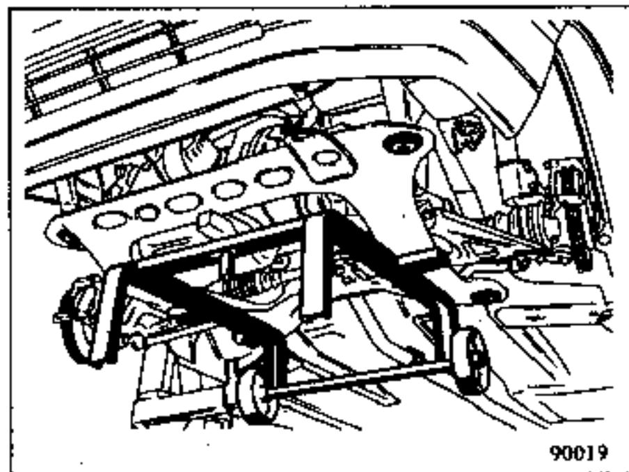
Lower the lift until the dummy frame makes contact with the floor.
