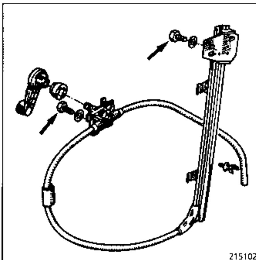
**Mechanism with window winder :**
