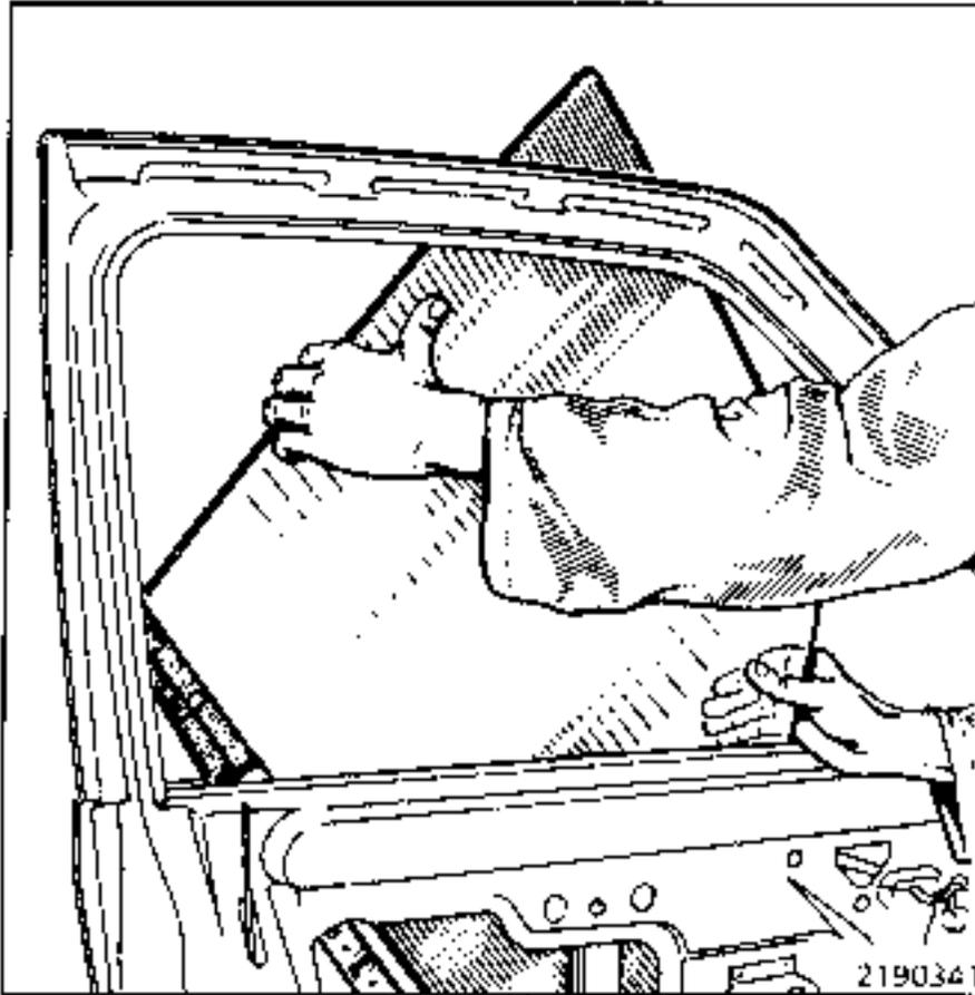
NOTE : The mechanism does not have to be replaced when replacing the window.
