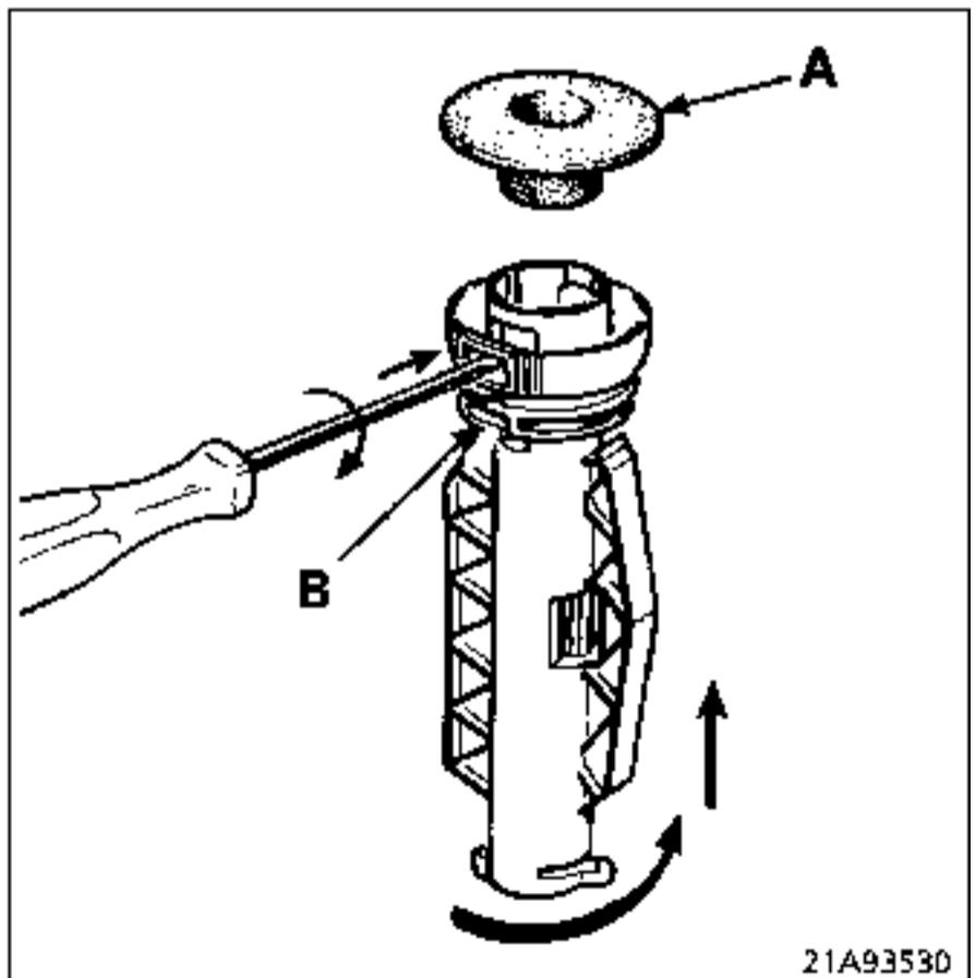
In order to remove the trim completely, unclip the two covers (A) from under the trim.
