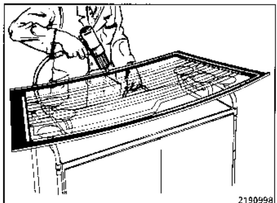
Using a spray gun, apply a bead of mastic to the primer strip, using the mouldings as a guide on the upper and lower edges..
