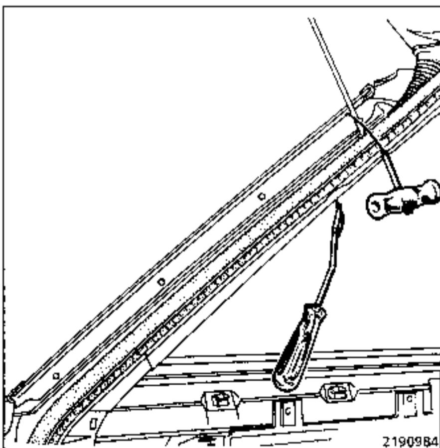
Using a wide strip of adhesive tape, protect the bodywork around the edge of the window.
