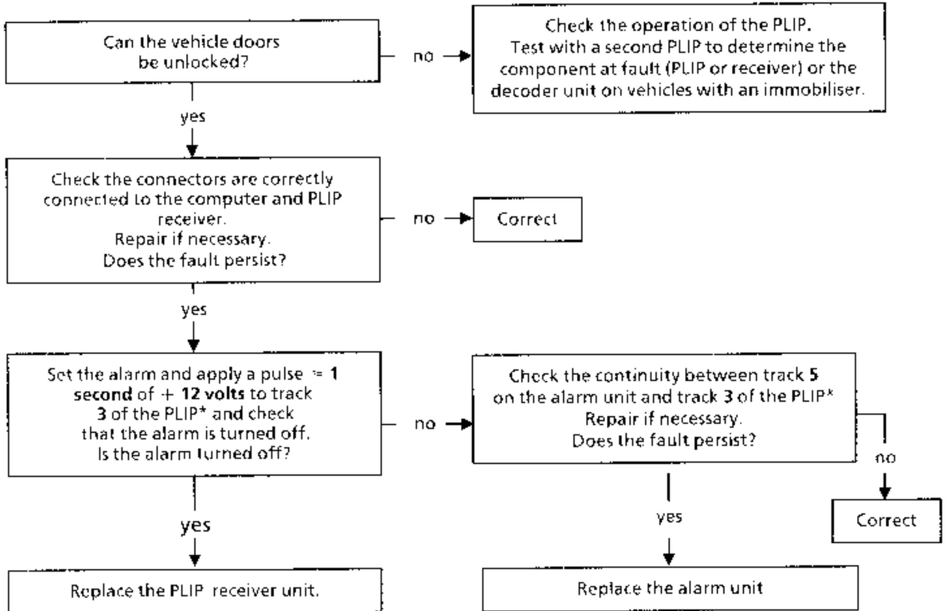
(\* ) track **A6** on the decoder unit for vehicles fitted with an immobiliser
