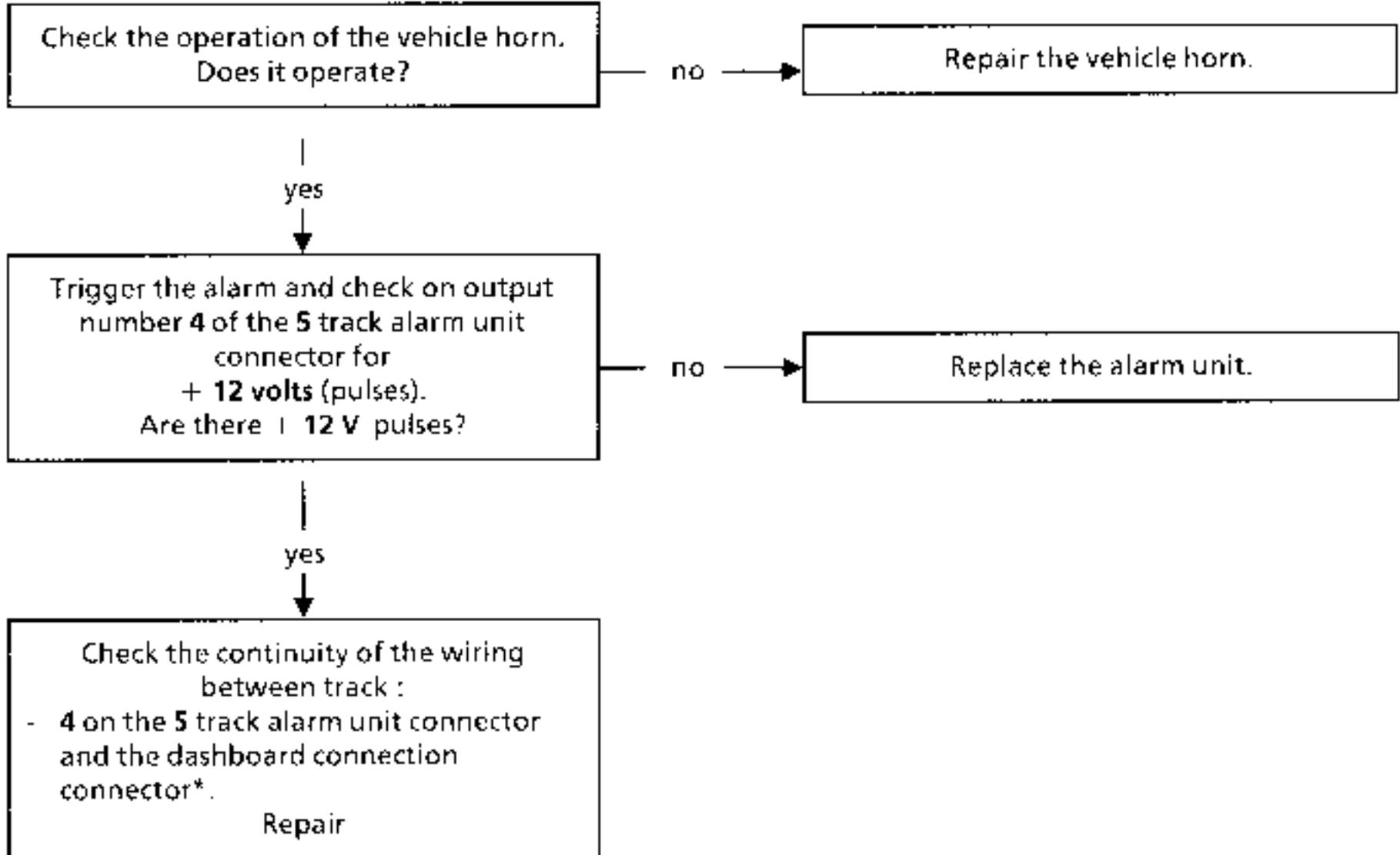
{\*} see vehicle wiring diagram
