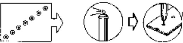
Four plug welds on each support (drill to diameter 5.5 mm).
