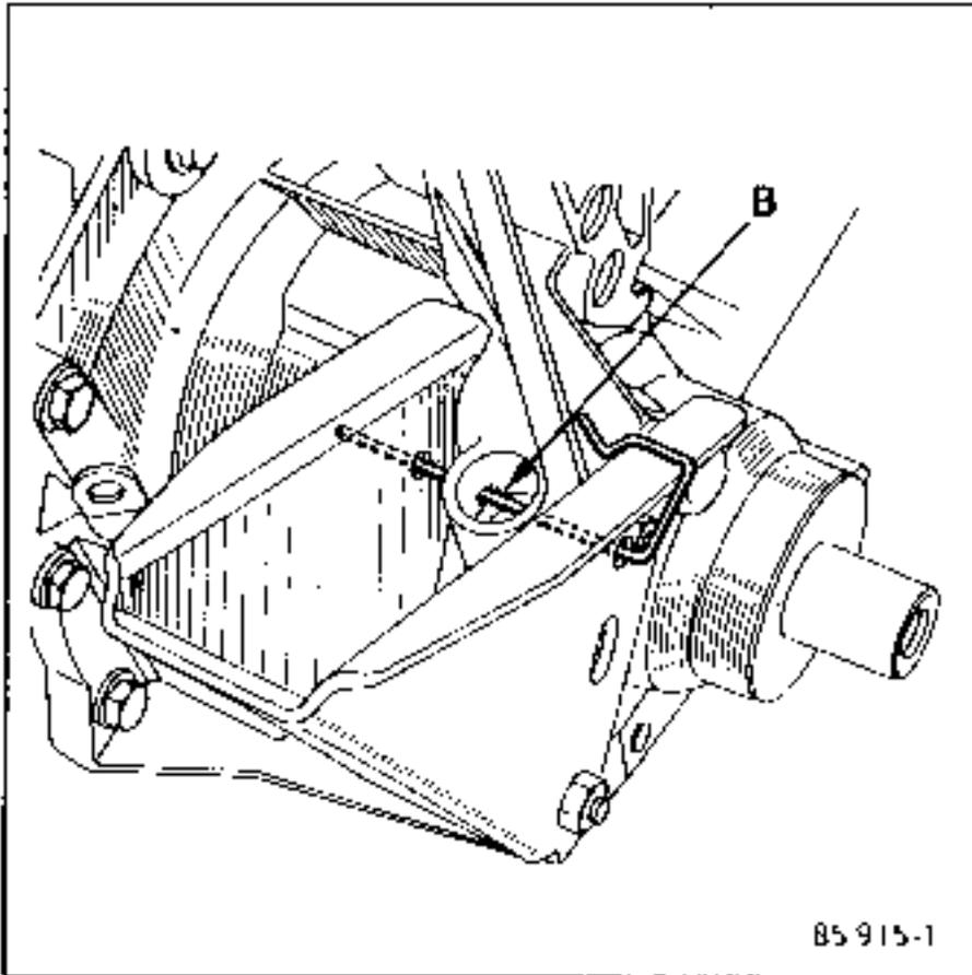
The steering column universal joint, bolt (1) after marking its position on the steering box.
