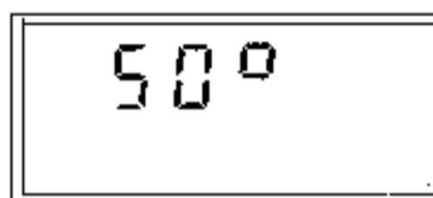
But the temperature is not **50°C**, it is an indication of a short-circuit on the thermistor or its wiring.
