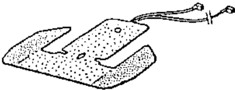
After removing the trim, carefully unstick the heating unit from the foam.
