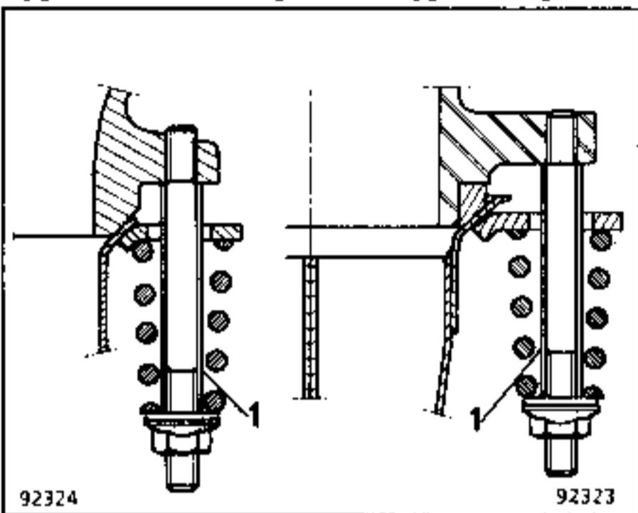
NOTE: the exhaust down pipes are fitted with spacers (1) which determine the spring pressure. Tighten until making contact with the spacers.
