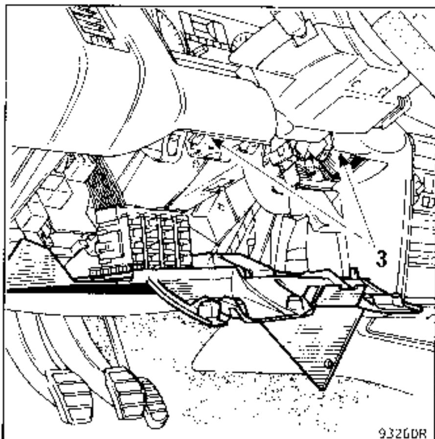
Lift the instrument panel fully up and remove it, whilst holding it raised.
