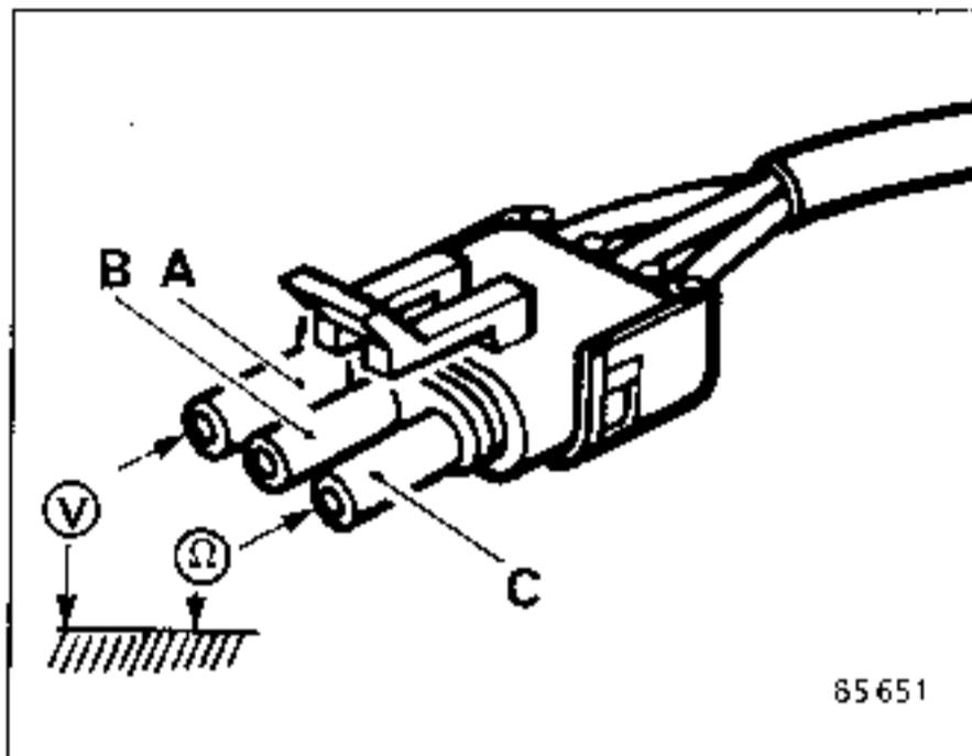
Disconnect the flow sensor and check :
