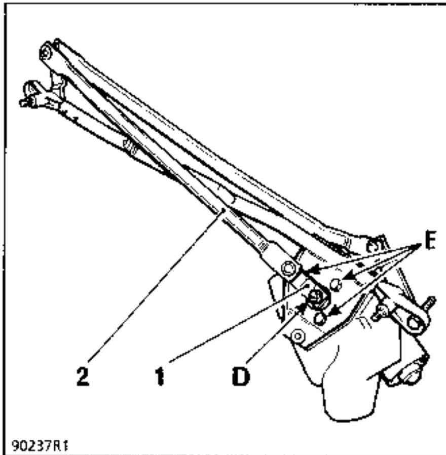
Unscrew securing nut (D) which secures the drive link (1).
