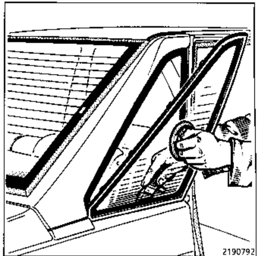
After the first two sides have been cut, move the window away and cut the remaining mastic using a cutting blade.
