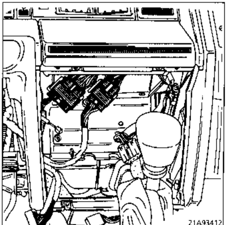
Disconnect the two connectors located on the air distribution unit.
