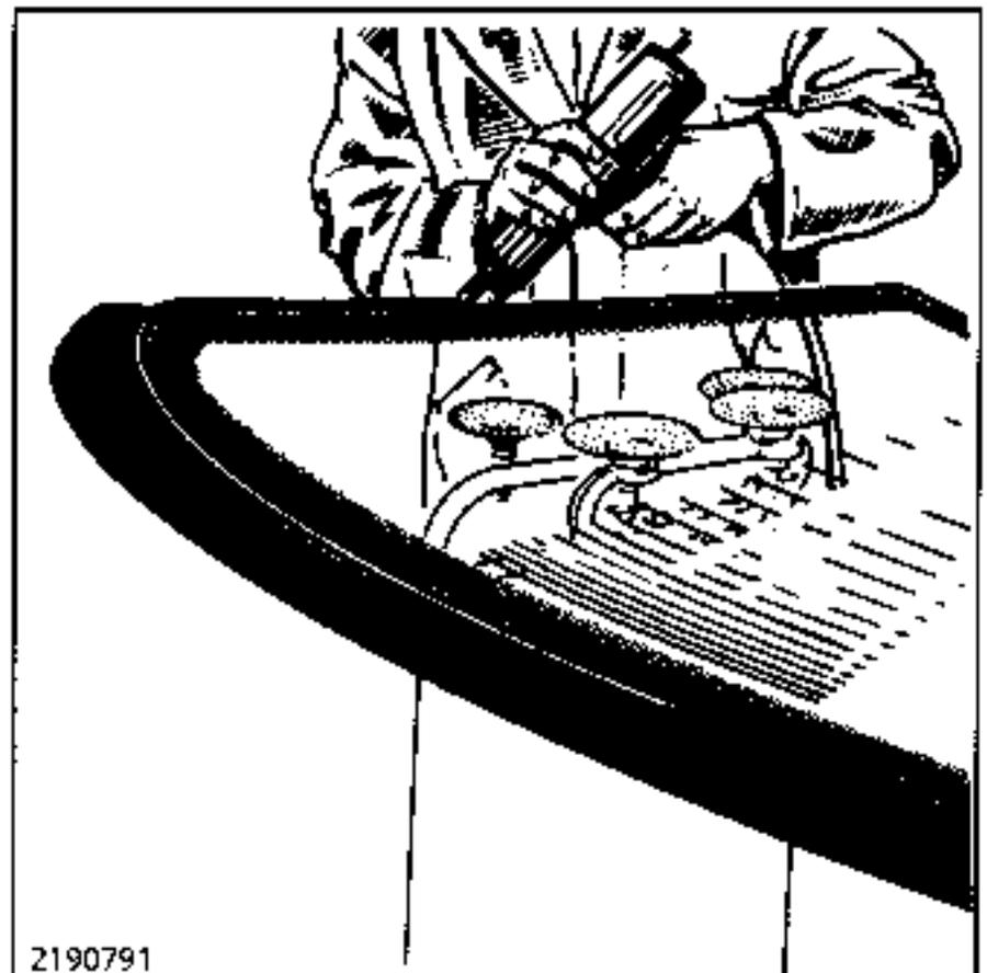
Using a spray gun, apply the mastic bead to the windscreen along the anti-overflow seal. Using a spatula, smooth down the join where the ends of the mastic bead meet.
