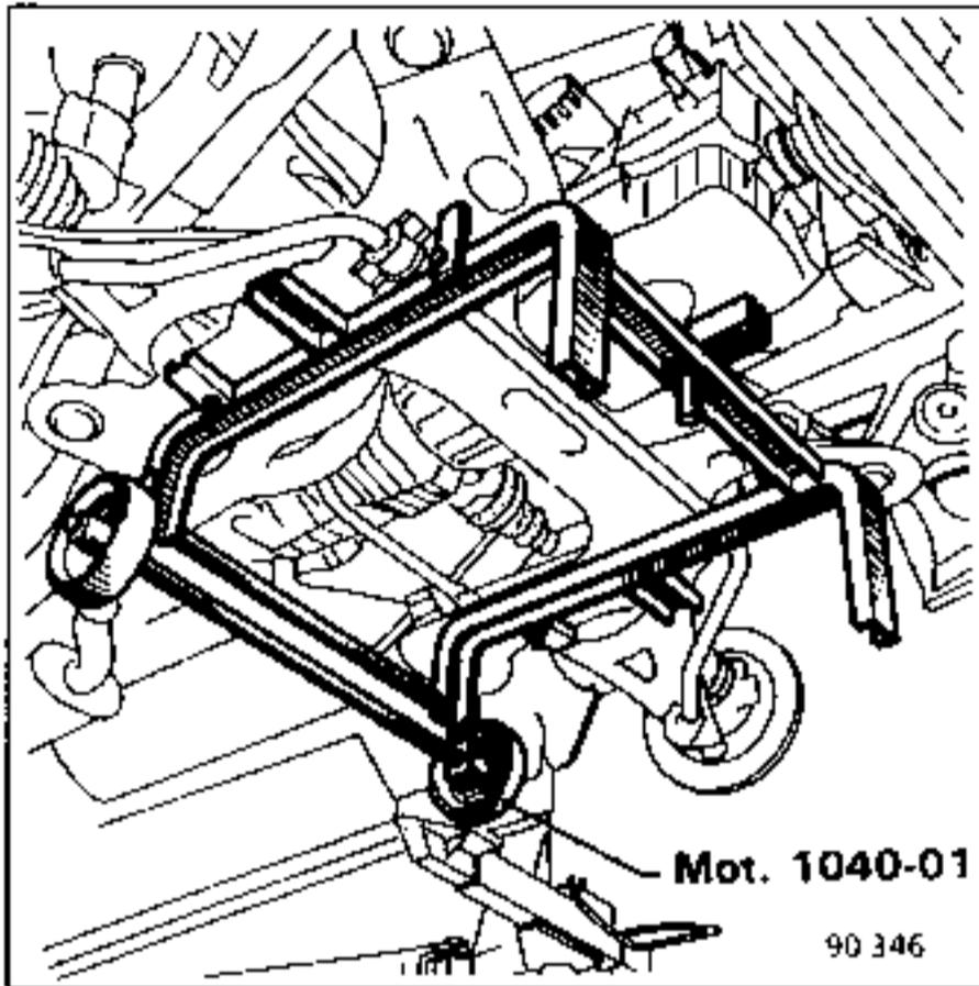
Lower the vehicle, fitted with sub-frame Mot. 1040-01, until it makes contact with the ground.
