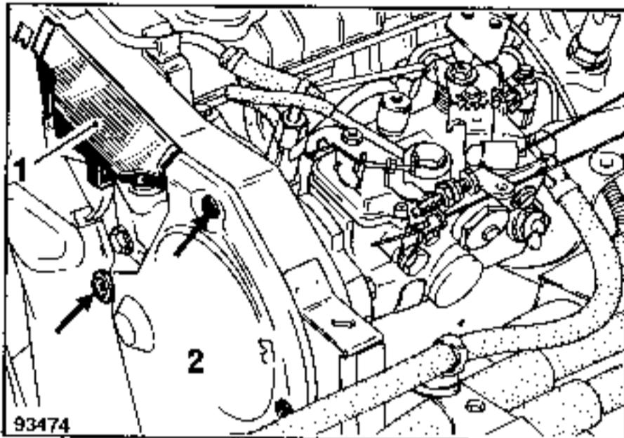
Remove the plastic cover (1) and the pressed steel casing (2).
