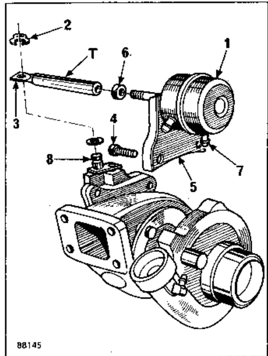
Place the new unit in position, securing it with new bolts (tightening torque 1.65 to 1.85 daN.m).
