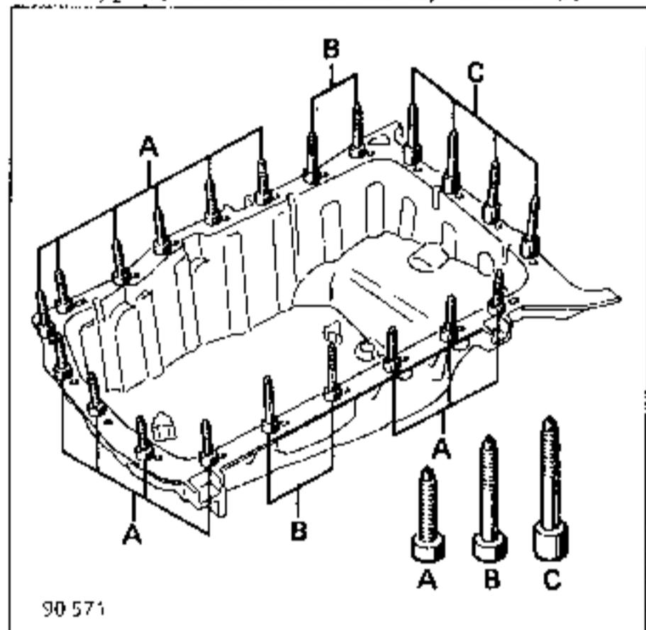
Do not refit the engine to the vehicle before tightening the sump screws.
