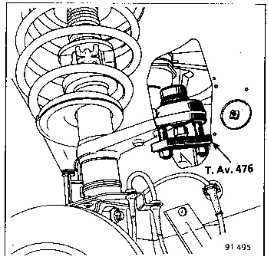
Knock out the spring pins from the drive shafts.
