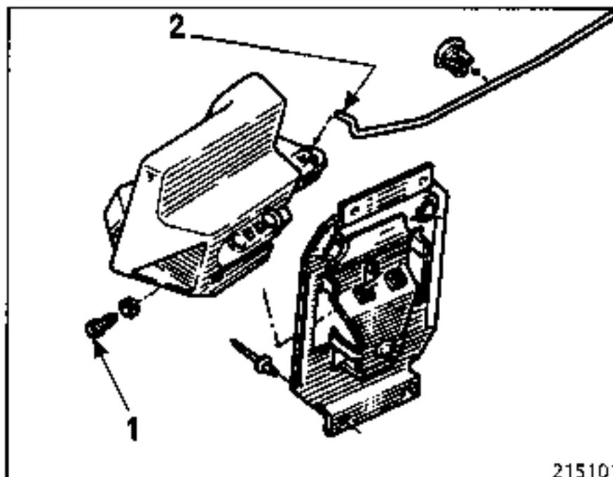
Remove screws (1) and separate the interior opening control from the linkage (2).
