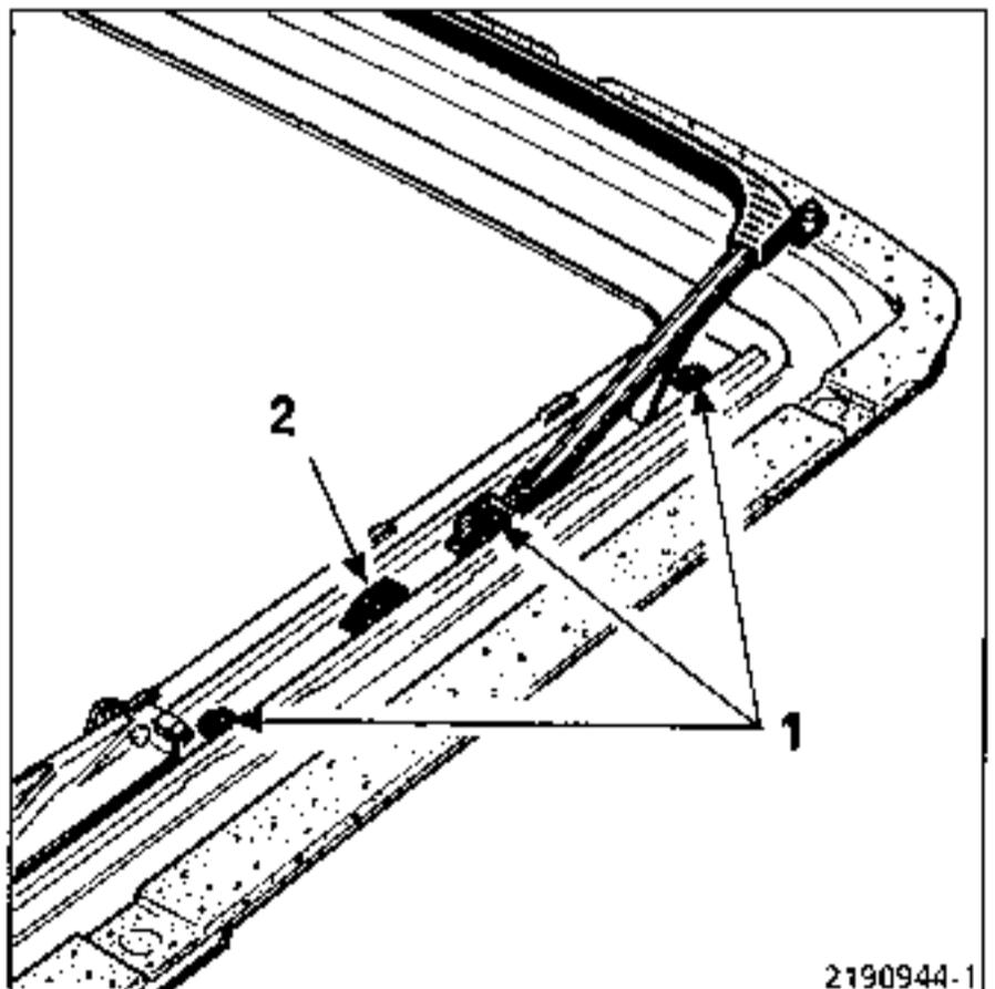
Move the mechanism into the "open" position.
