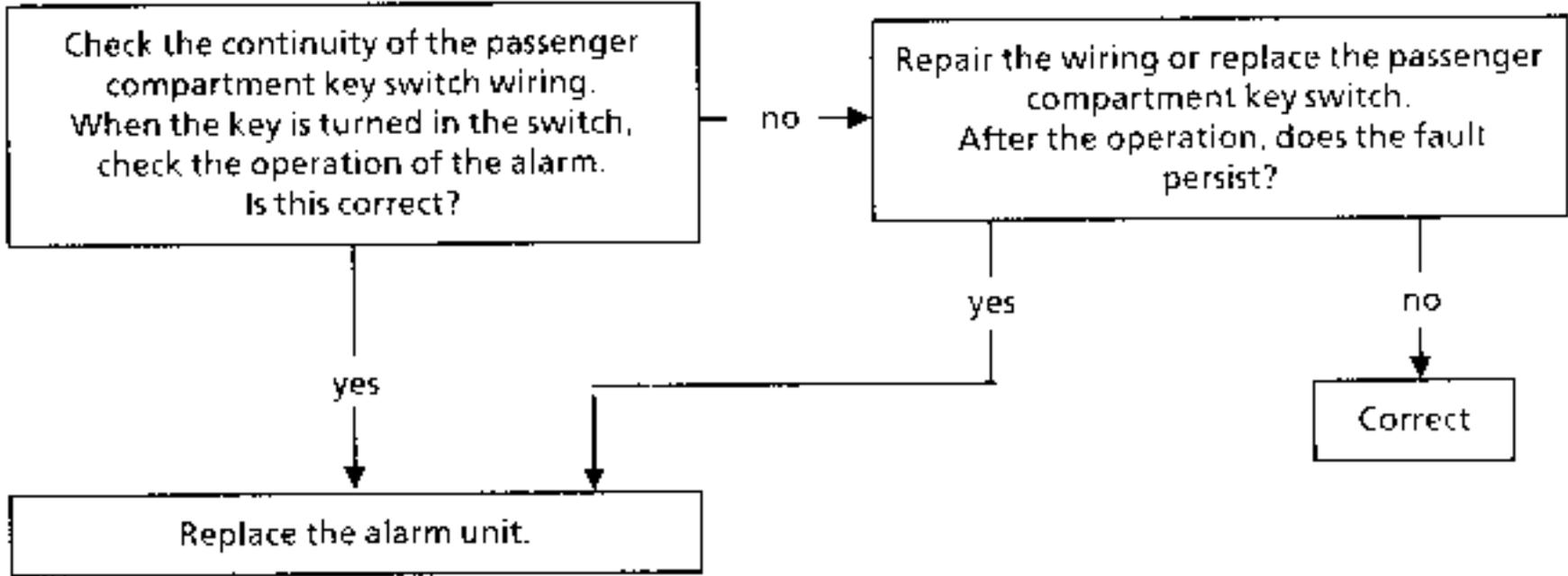
Chart 4 : Alarm triggered incorrectly when on stand by
