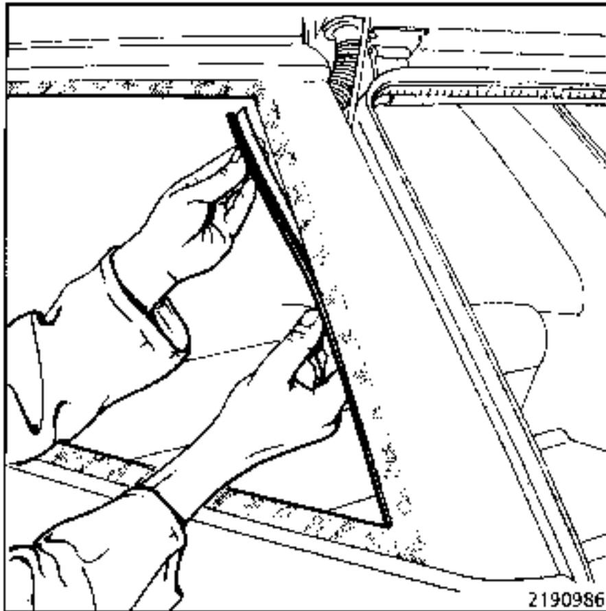
Fit the anti-overflow seals (1 per side), sticking the adhesive surface inside the aperture.
