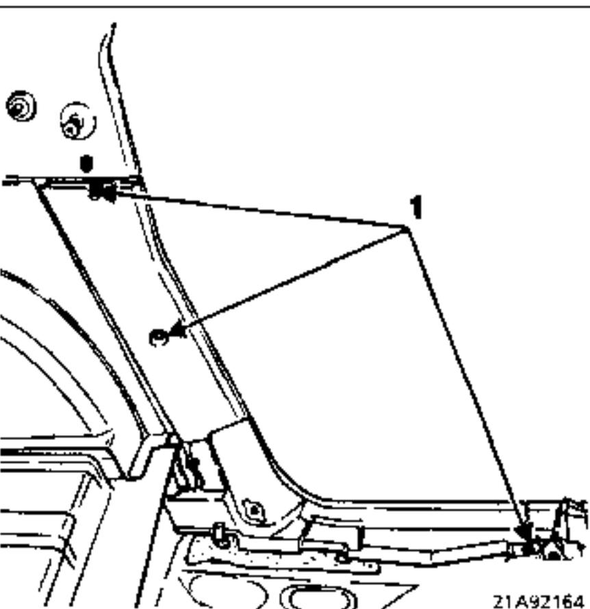
Remove the lower mounting for the seat belt.
