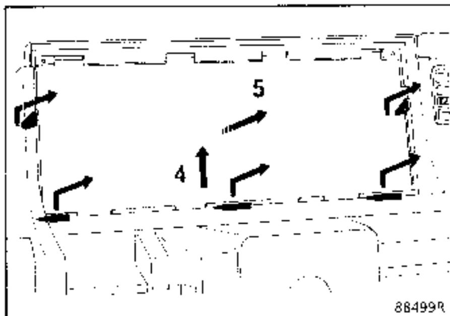
Remove the instrument panel (5) whilst holding it up to free the lugs (6).
