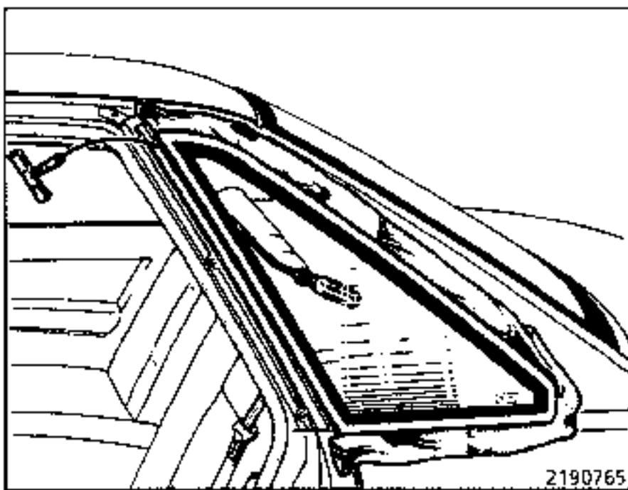
Pass a piece of steel wire approximately 30 cm long through the bead of mastic at the upper corner. Fit in place the pricker tool and pulling handle. Cut the mastic bead following the order shown in the drawing.
