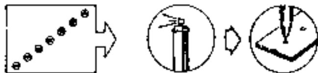
Plug welds joining 3 thicknesses
