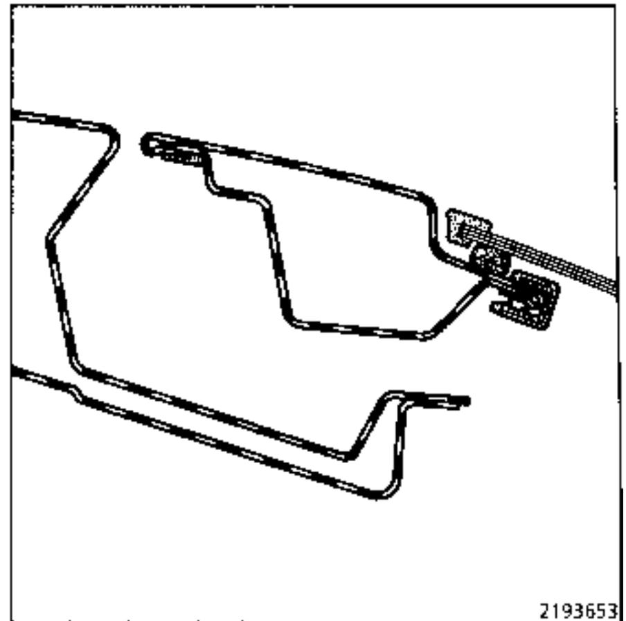
At the edges (lower and upper) check to see whether the clearance between the moulding and the surround is sufficient to pass through the cutting wire. If it is not, use Method 2.
