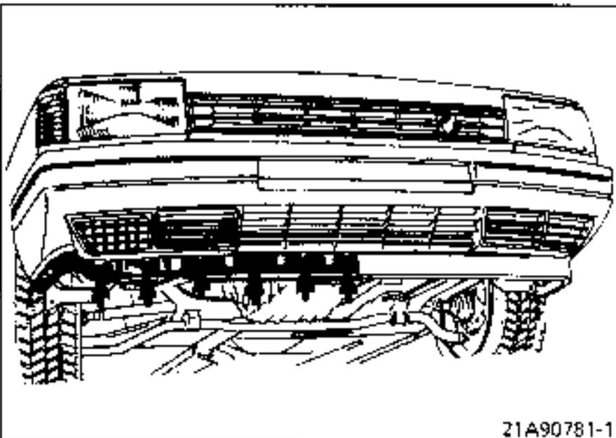
Secure the ends of the spoiler using mountings (2).
