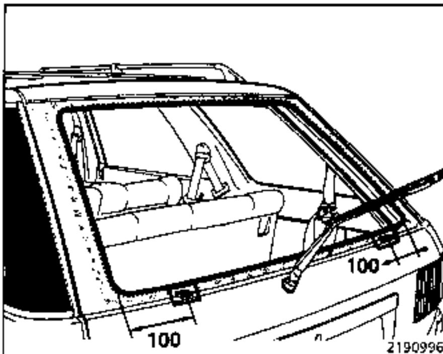
Using a rubber mallet tap the anti-overflow seal onto the screen surround (with the clips on the outside of the vehicle).
