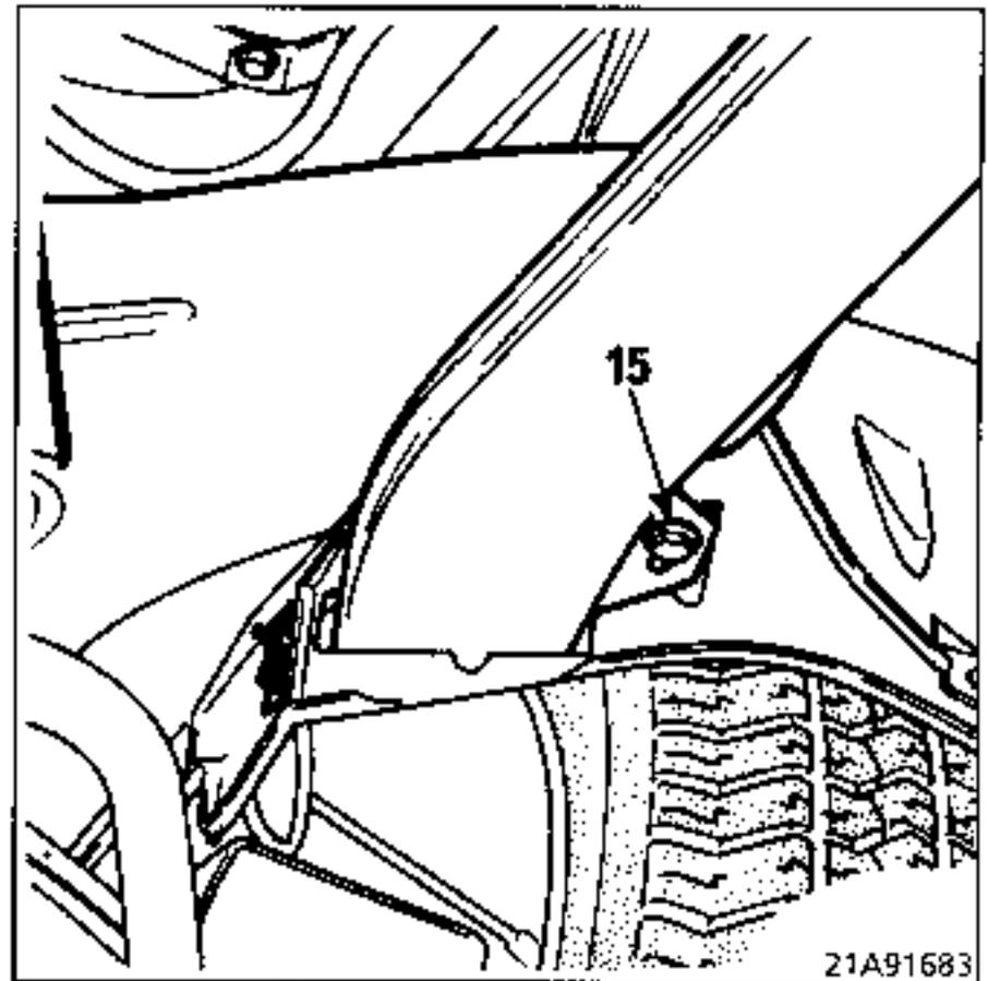
Secure the rear part to the protective shield using bolts (15).
