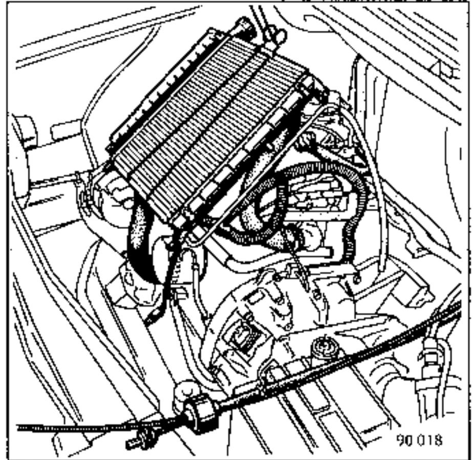
Fit the 2 clamps Mot. 453-01 to the heater hoses, then disconnect them from its inlet and outlet sides.
