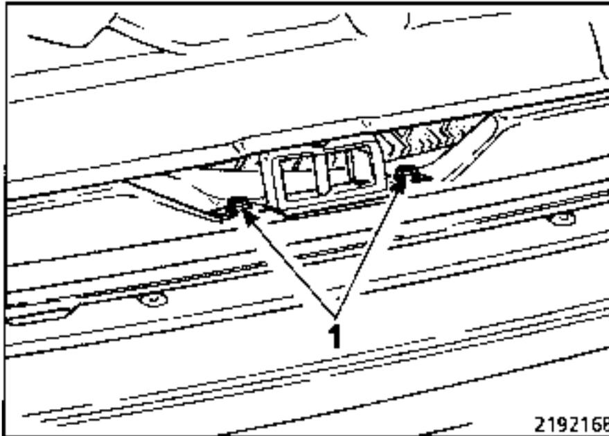
Use the two screws (1) to secure the striker plate in the desired position.
