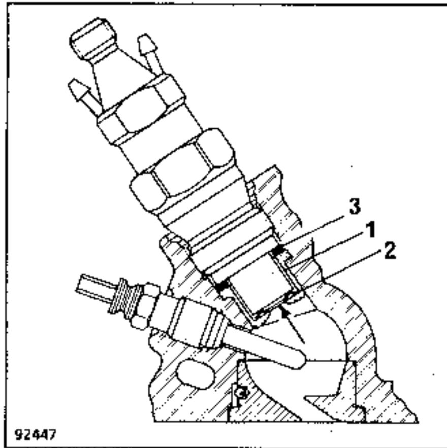
Each time an injector holder is refitted, fit a new seal (3) and a new flame baffle washer (2) (positioned as shown by the arrow).
