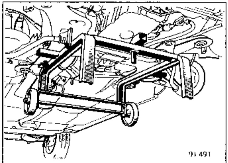
Lower the lift until the dummy sub-frame makes contact with the floor.
