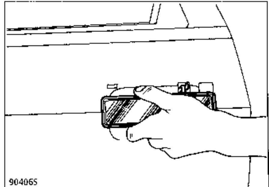
Using your thumb, push the clip on control rod (2) downwards and take the upper end of rod (2) out of the door panel.
