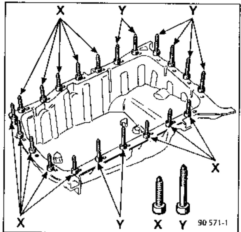
The screws are of the Torx type and tool Mot. 1 063 must be used.
