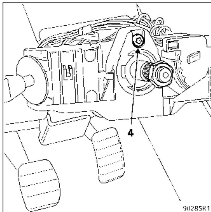
Unscrew screw (4) without removing it, then push it back to free the clamping taper.
