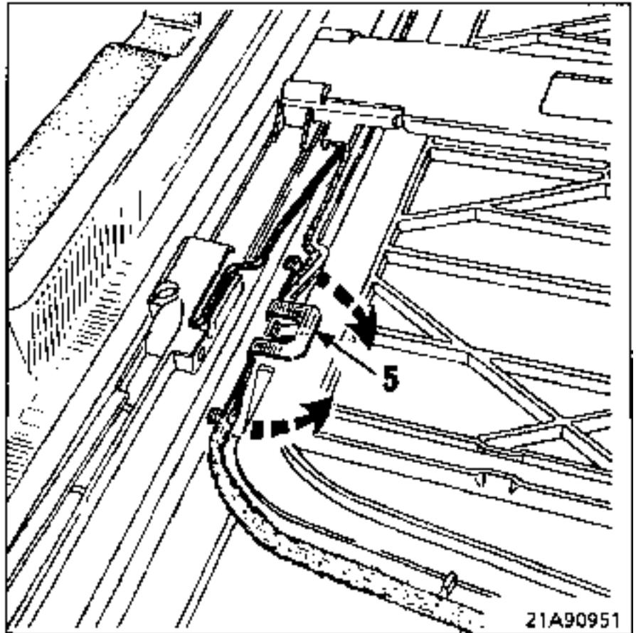
Using a screwdriver, free the guide springs (5) from the rails and remove the screen.
