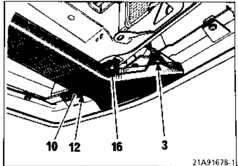
Offer up the air ducts and secure them using rivets (12) on lugs (10), screws (16) on the lower cross member and screws (3) on the spoiler.
