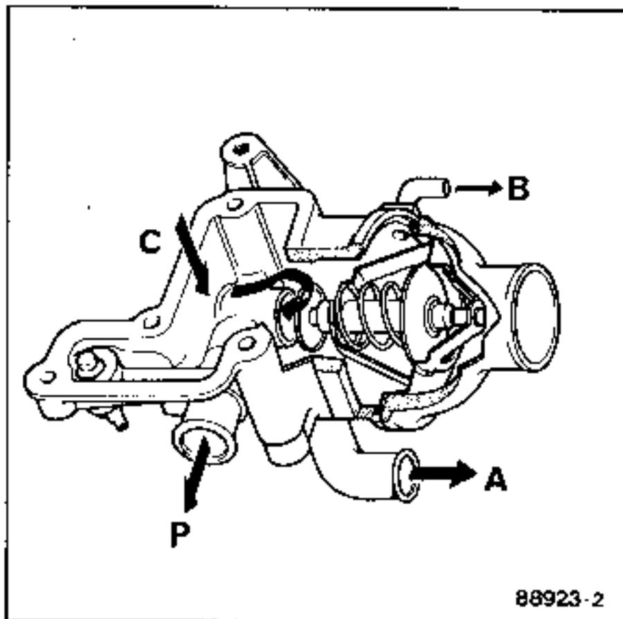
The thermostat (Figure 1) is closed and the coolant from the cylinder head (circuit C) is passed back to the coolant pump through circuit P, the heater through circuit A and the cold starting system (Bosch pump) followed by the "hot" expansion bottle through circuit (B).
