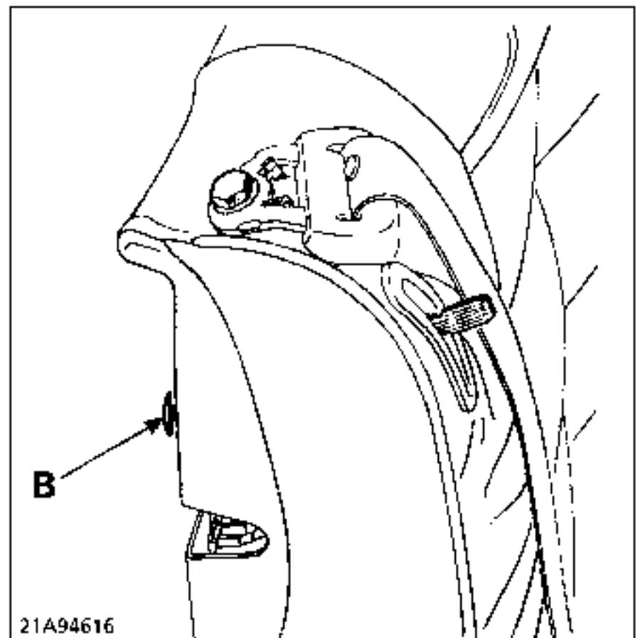
Remove the locking cover clips (B).
