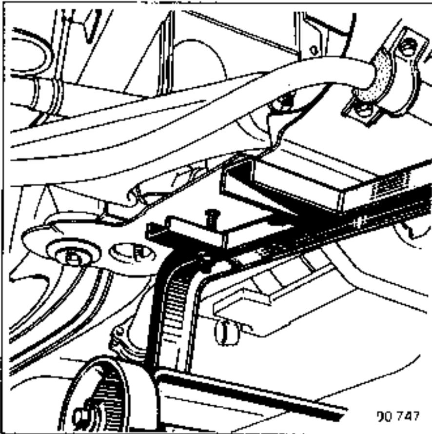
Remove the securing bolts from the shock absorber upper cups,
