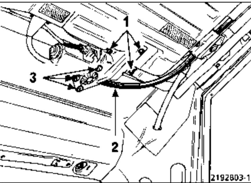
Disconnect the power supply connector from the motor.
