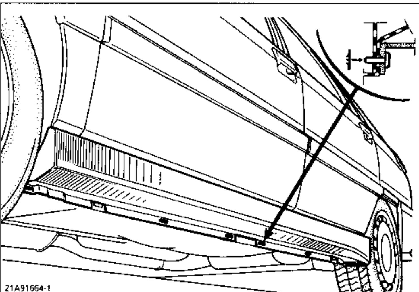
The skirt is removed by unpicking the lower plastic pins and pulling the skirt towards the front of the vehicle.
