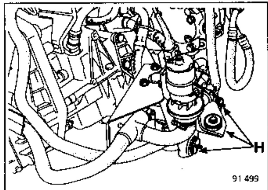
Fit the 2 clamps **Mot. 453-01** to the power steering reservoir output hoses.
