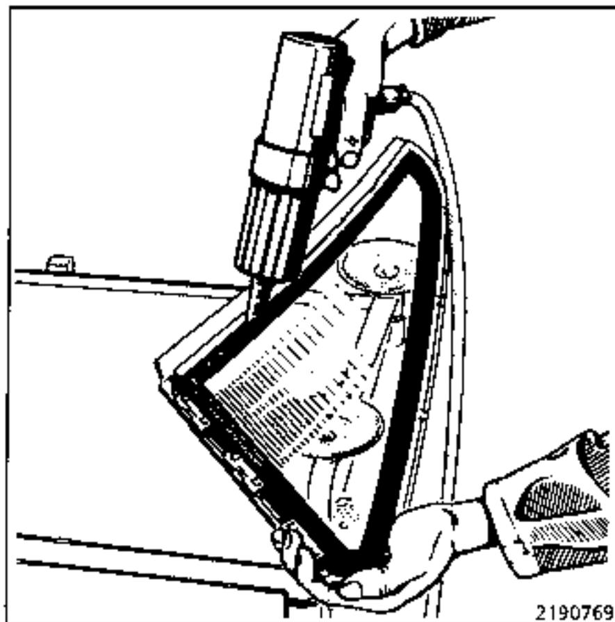
Using the spray gun, apply a bead of mastic to the window running along the edge of the clips and following the edge of the moulding frame. Use a spatula to smooth down the join where the ends of the mastic bead meet.
