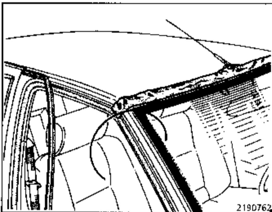
At one of the upper corners pass a piece of steel wire approximately 30 cm long through the mastic bead.
