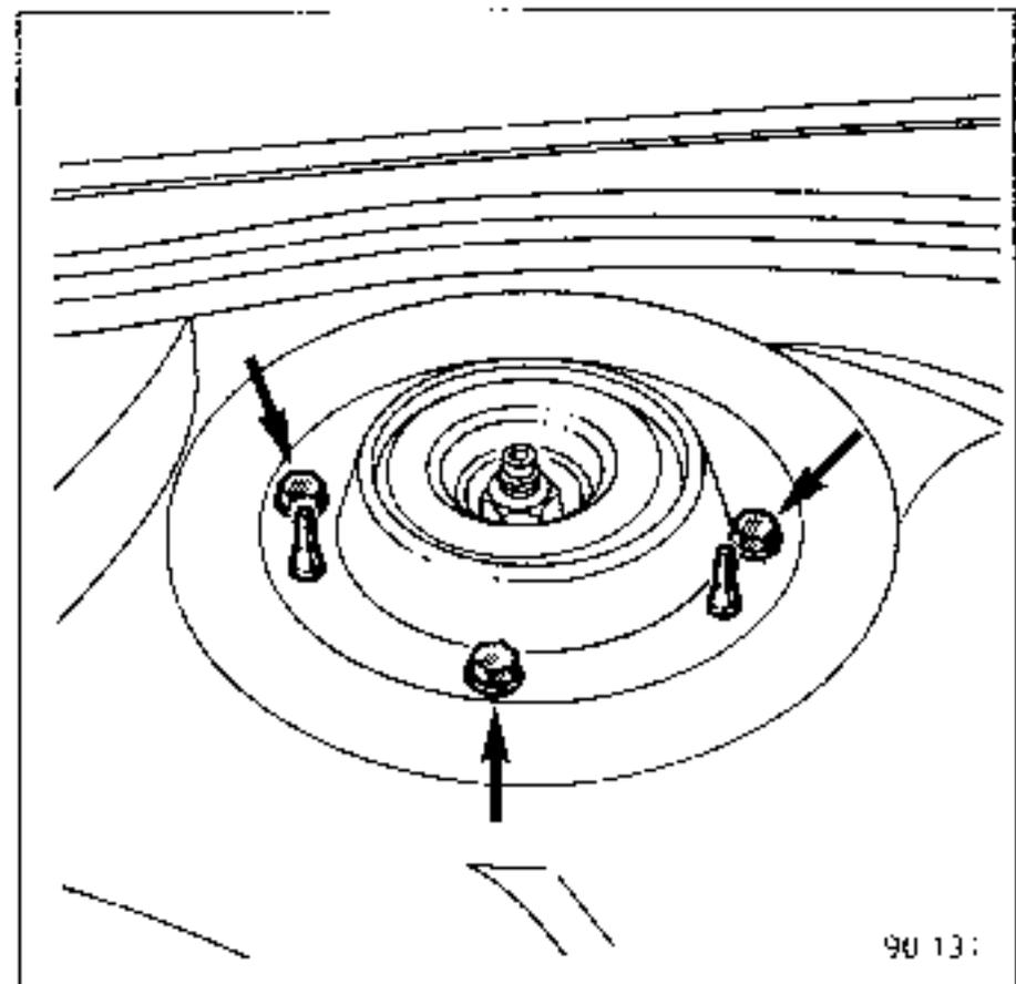
Remove the nut from the suspended flexible mounting and free the screwed rod from the flexible bush by knocking it with a bronze drift.
