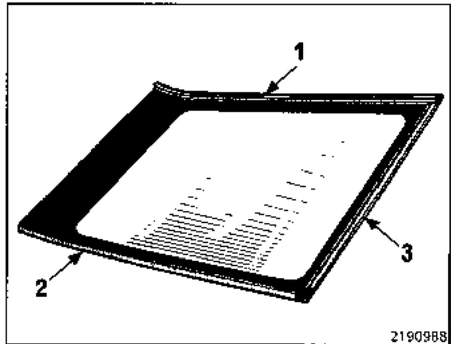
Fit the upper and lower trim pieces (1) and (2) to the edge of the window pushing them down to approximately half the depth of the U shape. Then fit the front moulding (3) in the same way.
