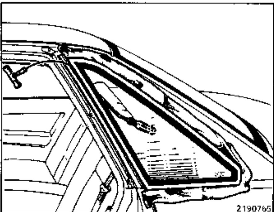
Pass a piece of steel wire approximately 30 cm long through the mastic bead at the upper corner. Fit in place the pricker tool and pulling handle. cut the mastic bead following the direction shown in the drawing.
