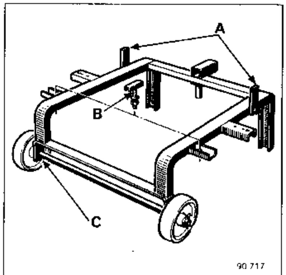
Secure frame Mot. 1 040-01 under the sub-frame.
