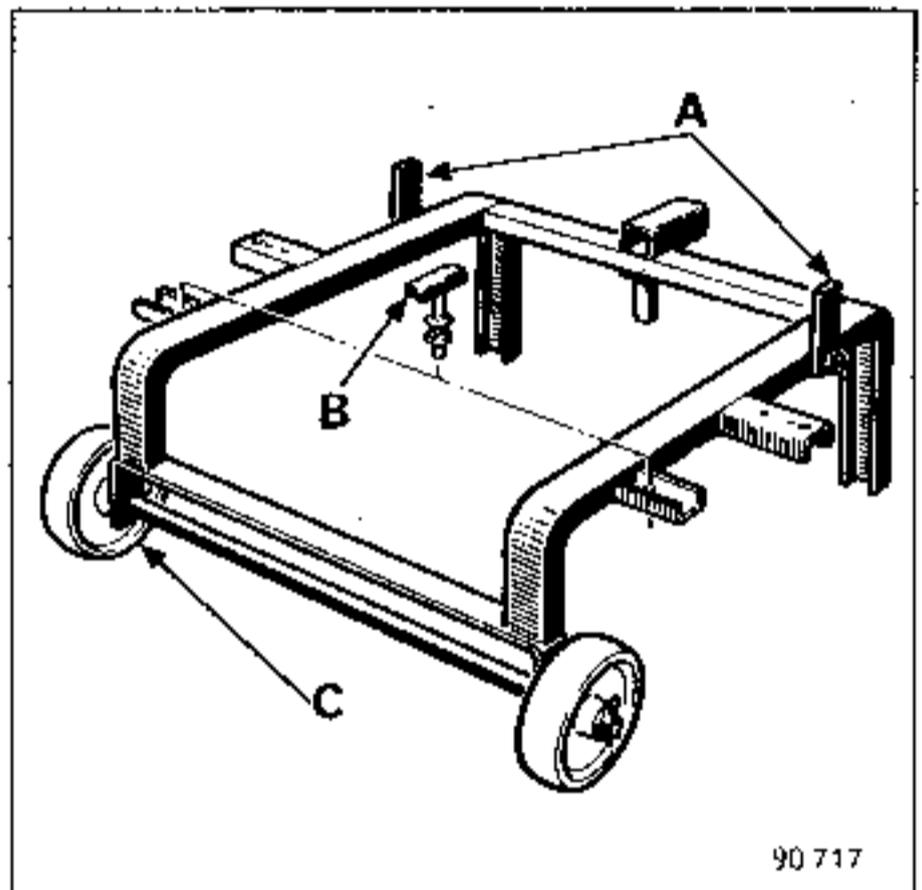
Secure the dummy sub-frame 1040-01 under the engine sub-frame.
