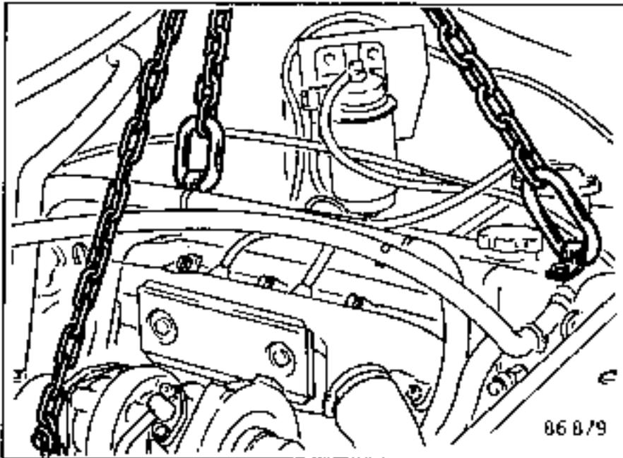
Lift out the engine-gearbox assembly
