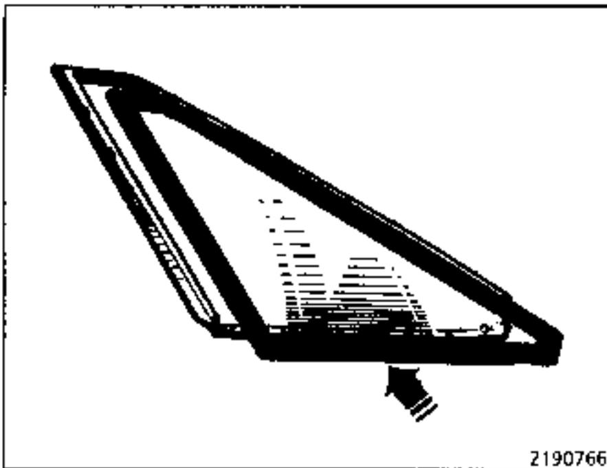
When the primer is dry, insert the window into the new moulding frame. Do not touch the prepared surface with your fingers.
