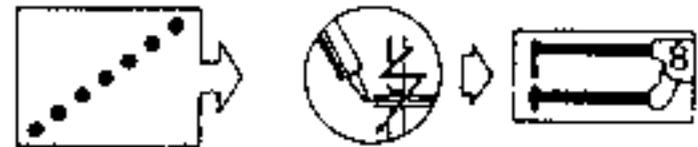
(A) 1 spot weld joining 3 thicknesses
