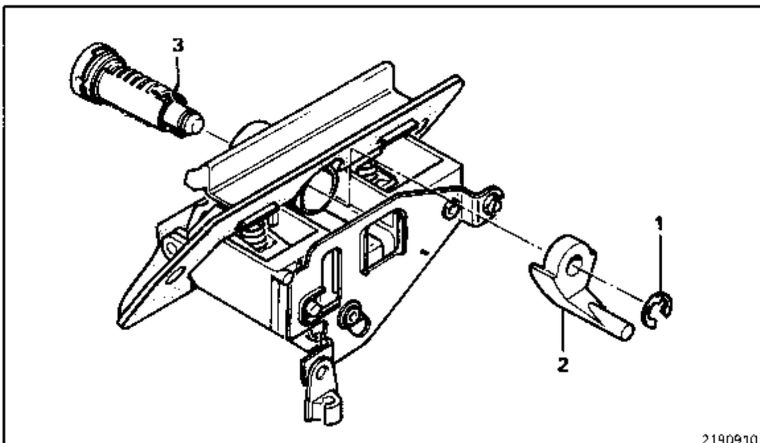
Remove clip (1), disengage control finger (2) and take the lock barrel out, moving it backwards.
