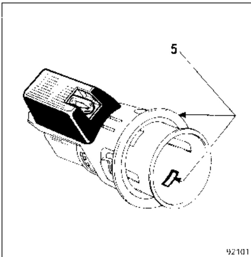
Take out the plastic part by pushing the back of it
