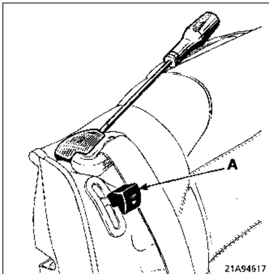
After removing the seat, remove handle (A).
