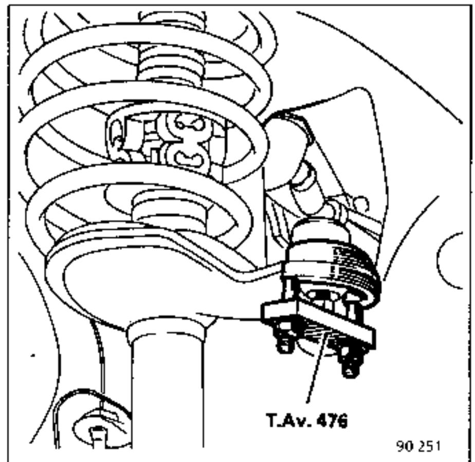
Remove the upper bolts securing the lower ends of the shock absorbers and loosen the lower bolts without removing them.
